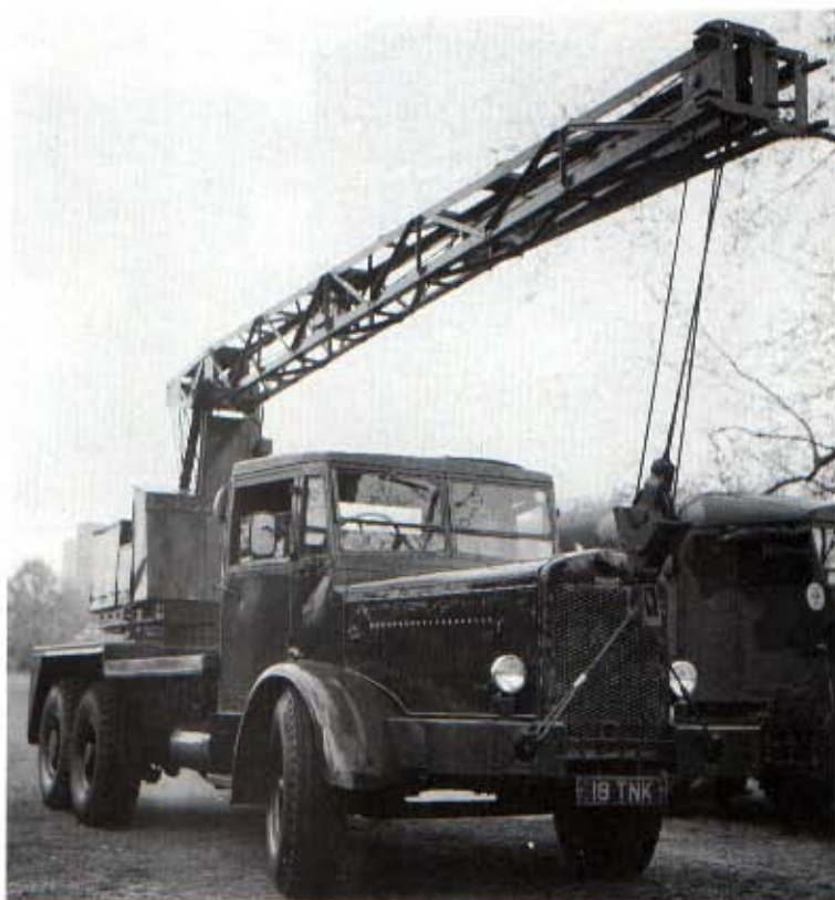
Above: Another popular chassis for crane carrying was the Thornycroft Amazon, which, like the AEC, used a Coles Mark VII. About 2000 were made during the war, of which the RAF took 1800. (NMM)
