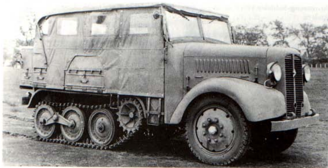
Left: Ikegai KO-H1 5-Ton halftrack tractor, intended as an AA gun tractor with a crew of fifteen. It was powered by a 110bhp six-cylinder diesel engine. (Bart Vanderveen Collection)
