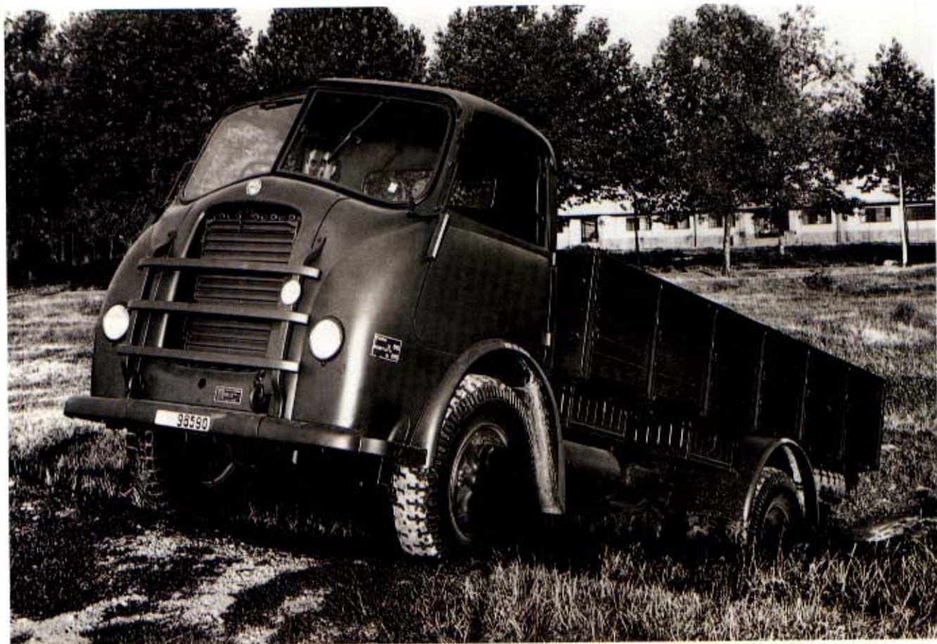
Above: An Alfa Romeo 800 8-ton truck which came into the AUP (Autocarro Unificato Pesante) heavy truck category. It used the company's own 8725cc diesel engine, and was made from 1940 to 1944, and for civilian use, from 1946 to 1950.
