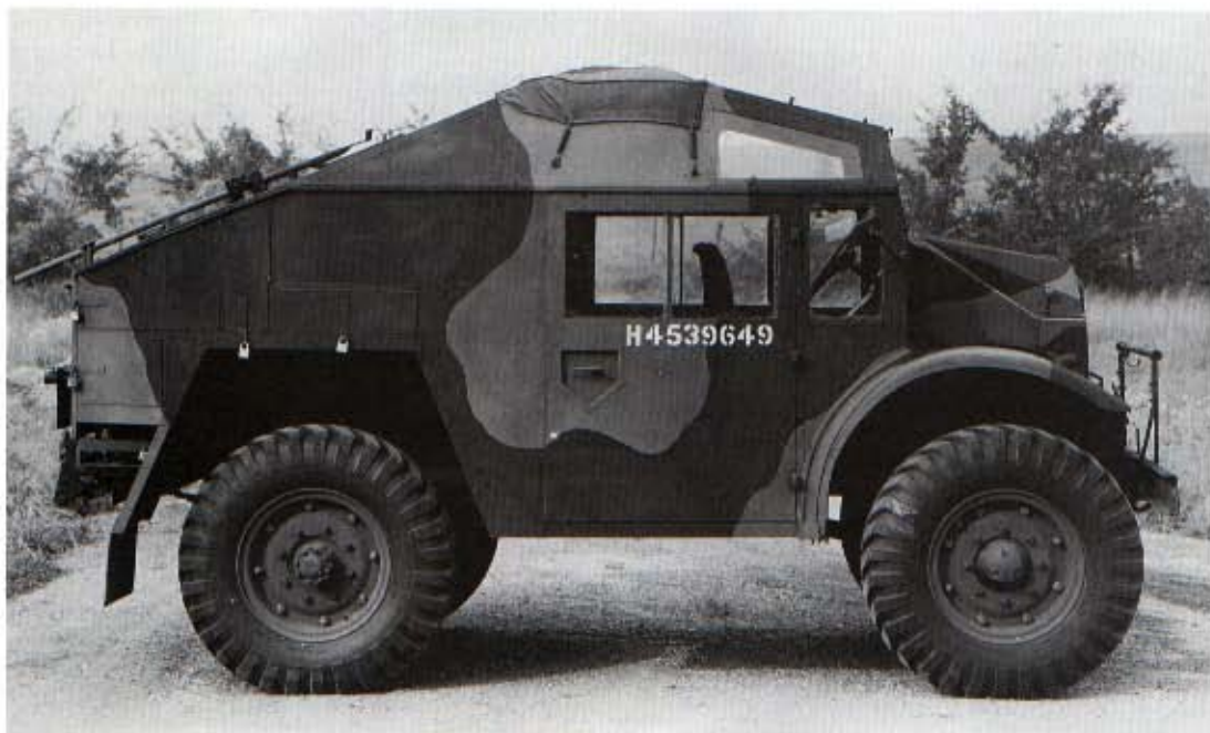
Left: The gun tractor on the 101in wheelbase was known to the Army as an FAT (Field Artillery Tractor), but in the makers' own terminology it was a CGT or FGT (Chevrolet or Ford Gun Tractor). This is an early type (pre-1942) CGT with the sloping roof cab of the Morris-Commercial Quads.
