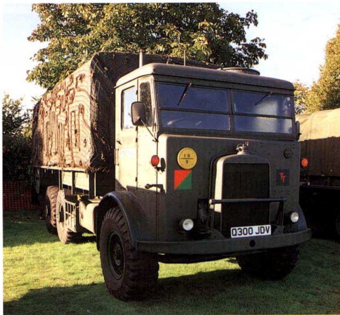
Right: The Leyland Hippo was one of the Army's 10-ton 6x4 trucks, the largest category of rigid chassis used by the British Army in World War Two. This is the Mark II, introduced in 1944 and made for several years after the war. Its 7.4-litre six-cylinder diesel engine developed 100bhp, and drove through a five-speed gearbox. (The Tank Museum, Bovington)
