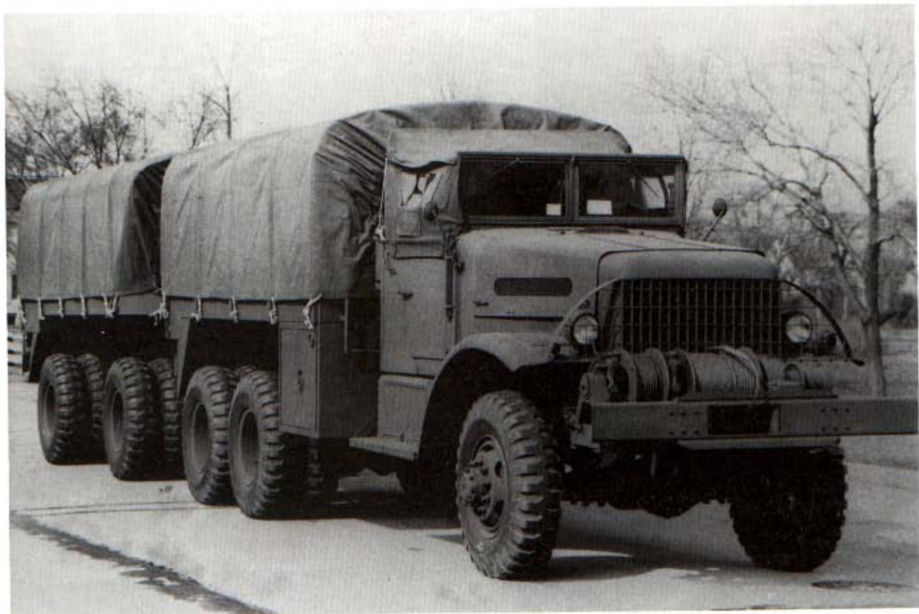
Above: This is a White 6x6, differing from the Corbitt in having a 25,000 pounds capacity winch ahead of the radiator, though this could be fitted to either make. The canvas top of the body and trailer concealed two 2000-gallon fuel tanks.
