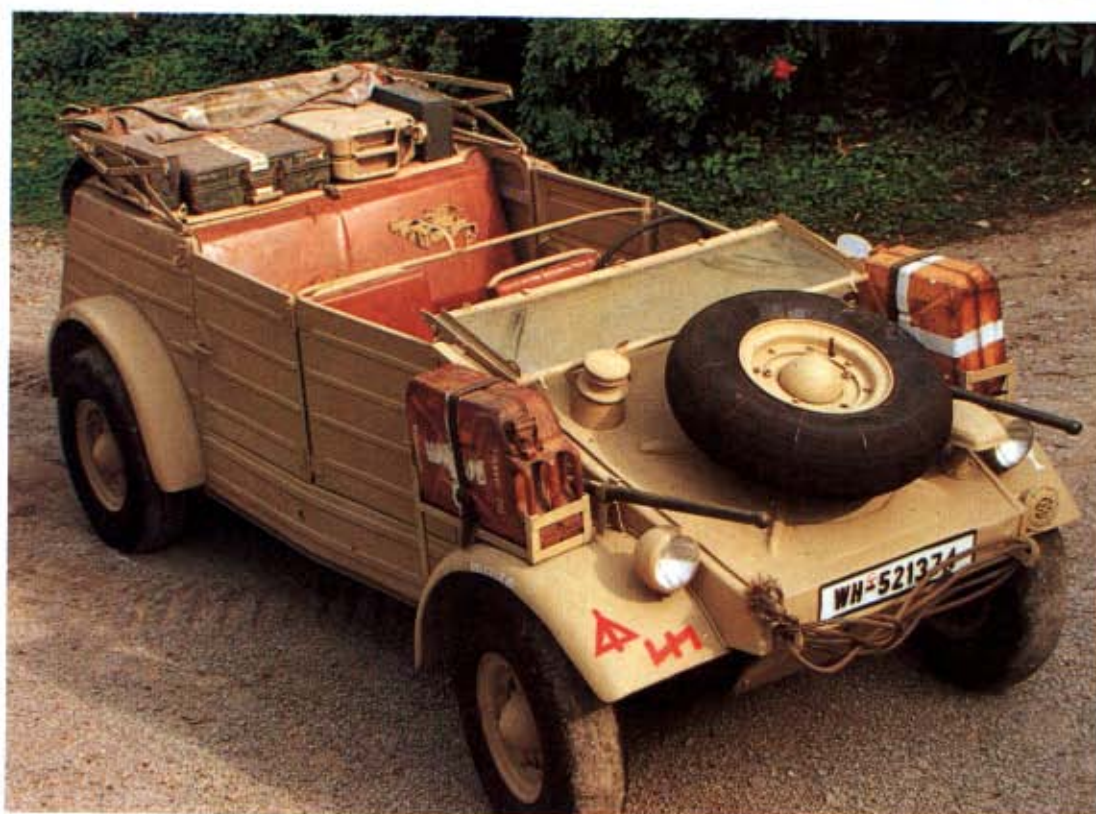
Left: Volkswagen's offering in the Kübelwagen field used the running gear of the familiar Beetle saloon. This one is in the insignia of the 21st Panzer Division, Afrika Corps. It has 690x 200 oversize tyres for desert use. (Vehicle displayed at the Victory Memorial Museum)
