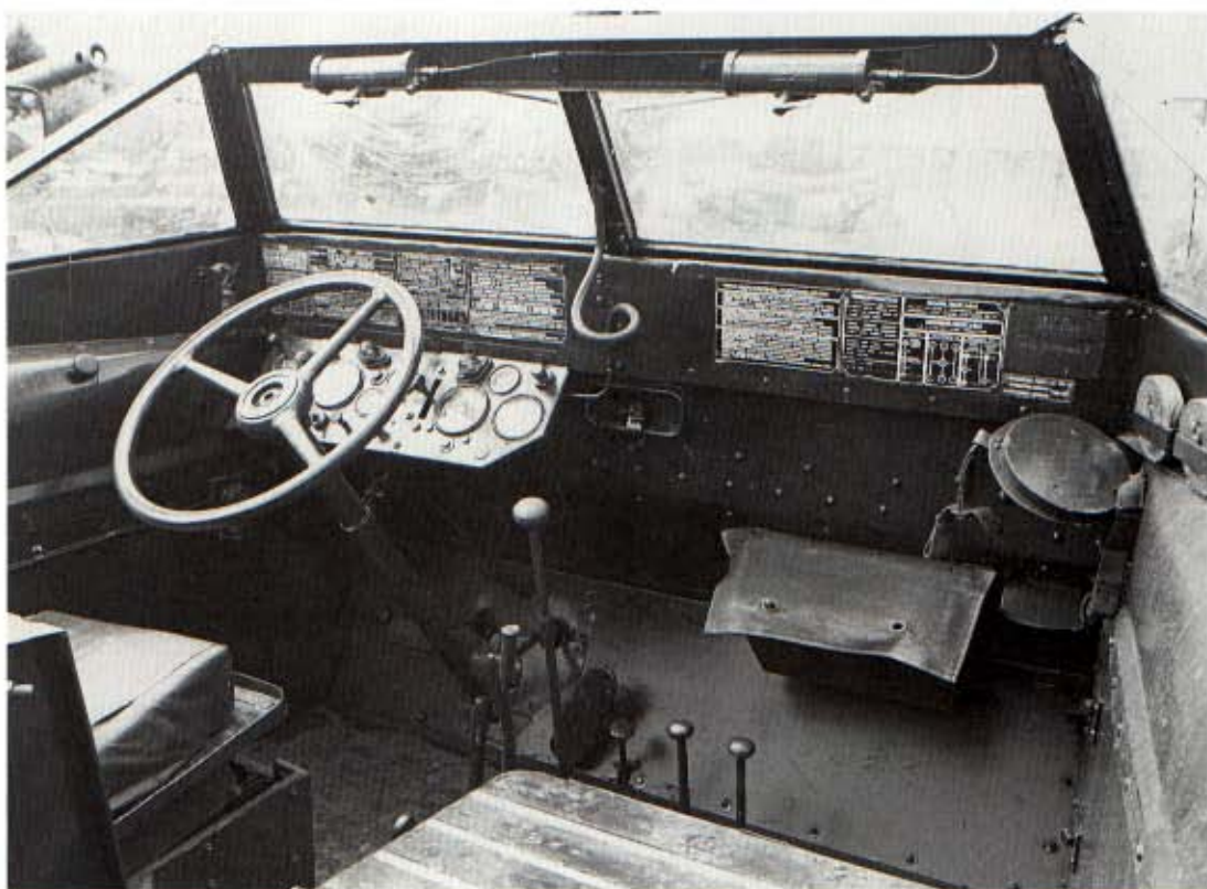
Right: Cockpit of a DUKW. The instructions on the right-hand side are about engaging and disengaging of the front axle. (The Tank Museum, Bovington)
