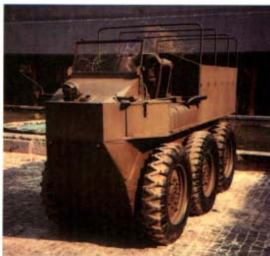
Below left: Only three Humber Hexonaut 6x6s were made, and this is the only survivor. It is powered by two Hillman 14hp engines, each driving the wheels on one side. (Vehicle displayed at the Victory Memorial Museum)
