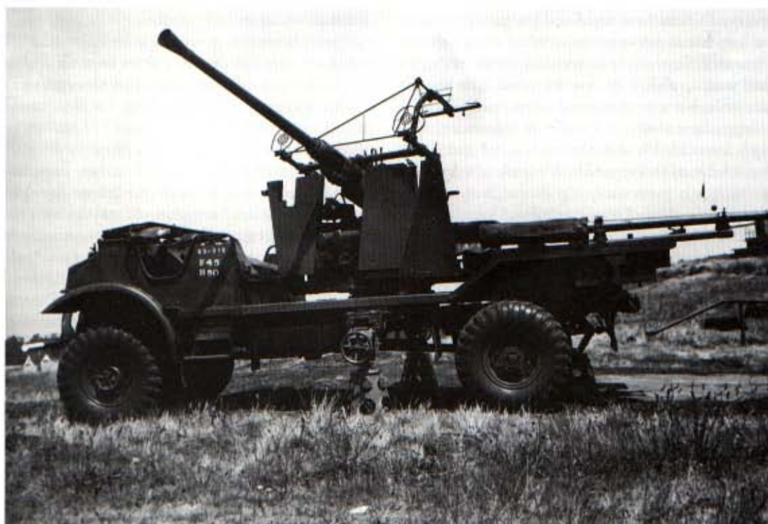
Left: A Ford F60B with 40mm Bofors AA gun on a reinforced chassis with an extra wide cab seating a crew of four. Though mainly for anti-aircraft work, the gun would be effectively used against ground targets. Projecting from the rear is a spare barrel. (Dr. William A. Gregg)
