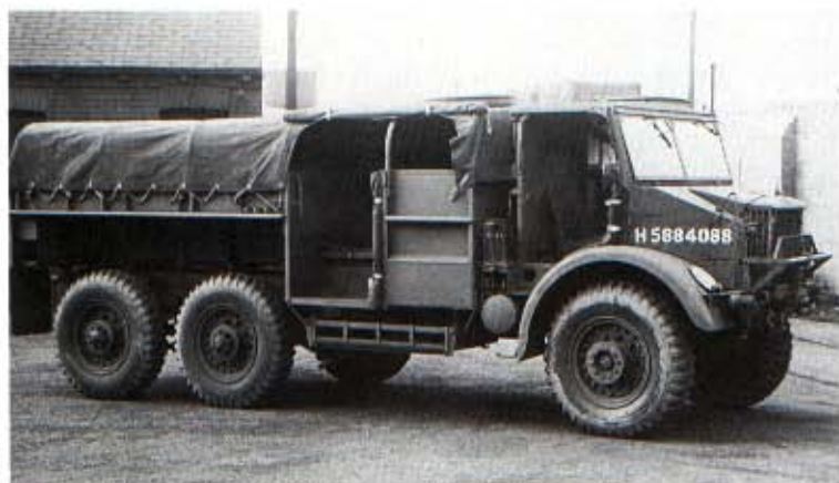
Above: Two Albion artillery tractors. Top is a CX225 6x4, powered by a 9.1-litre six-cylinder engine, of which more than 500 were made between 1943 and 1945. Bottom is a low-profile tractor, the FT15N; this was a smaller vehicle with a 4.6-litre engine and weighing 13,215 pounds, as against the 23,380 of the CX225. The FT15N had six-wheel drive and hydraulic brakes. Production did not start until January 1945 and continued until March 1946. (The Tank Museum, Bovington)
