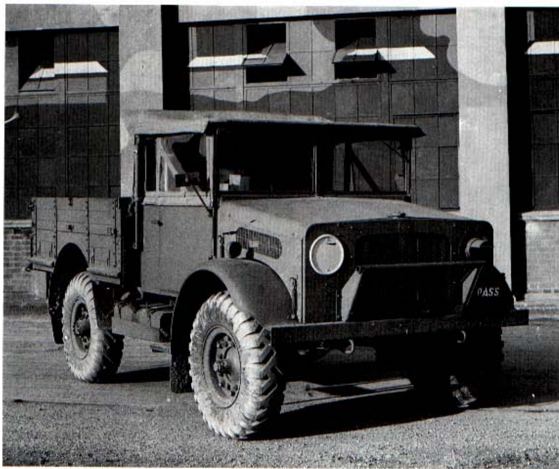
Left: The standard Bedford MWD 15cwt truck in its most familiar form. Earlier versions had twin aero screens which gave very poor visibility when the cape cart hood was erected. MWs were used by all three services, and were purchased in bulk by the Ministry of Supply, who then allocated them to the Army, Navy or Royal Air Force. (NMM)
