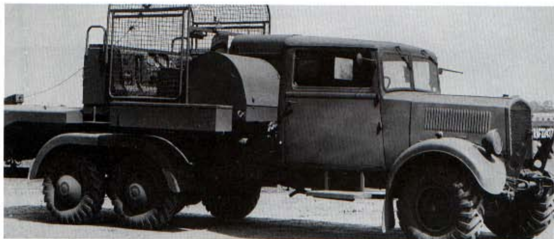
Left: Three chassis were favoured for barrage balloon winch duties, the Dodge 3 ton, Austin K6 and Fordson WOT1. This WOT1 carries a Wild winch Mark IV, and would have been used in conjunction with hydrogen cylinder trailer. Originally the winch lorries were kept at static sites, but the advent of the V1 flying bombs in 1944 necessitated the rapid deployment of balloons at different sites.
