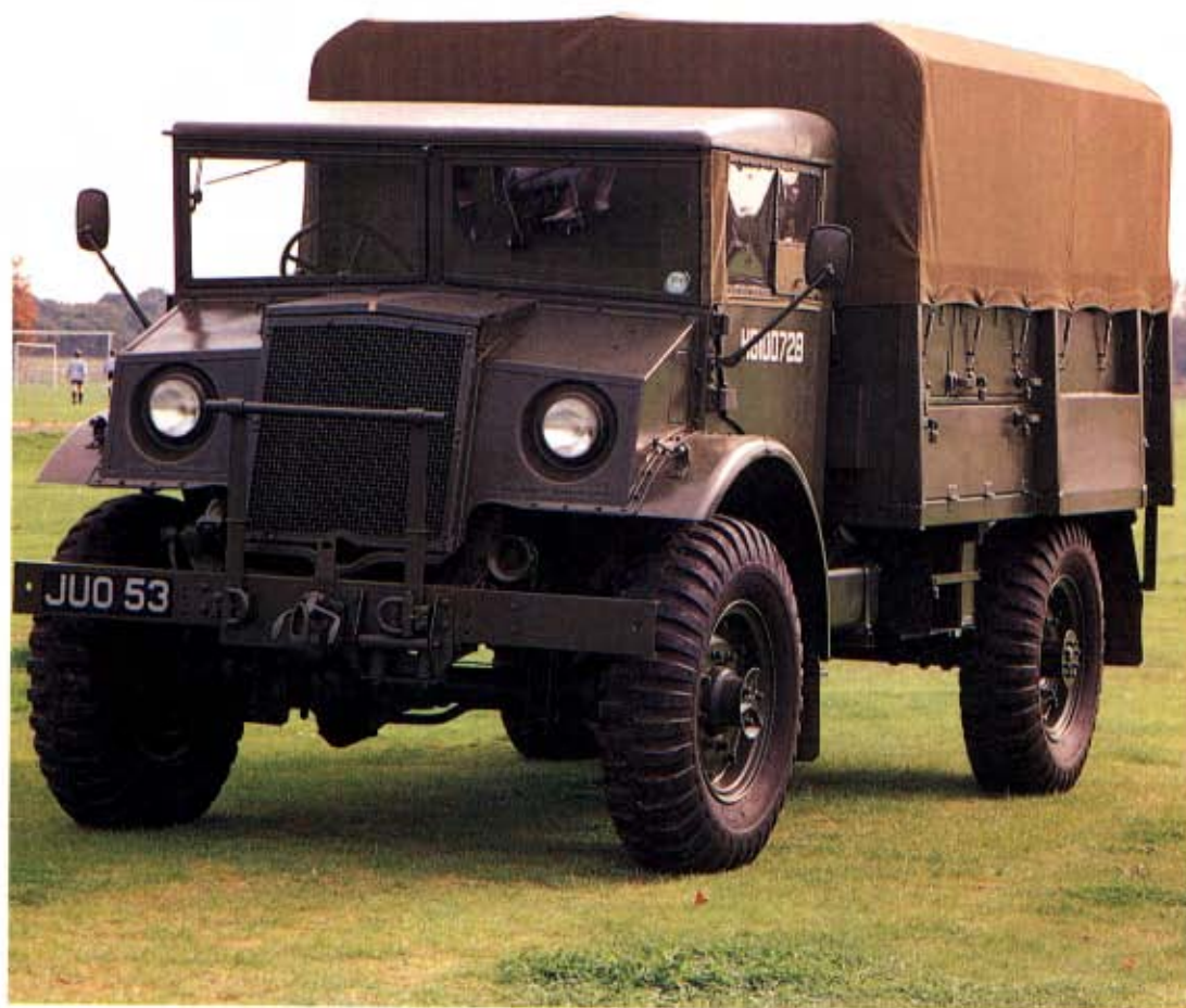
Left: This Ford-built CMP 3-tonner is an F60S (F=Ford, 60cwt S=short wheelbase). The wheelbase was 134 inches, compared with 158 inches for the F60L.
