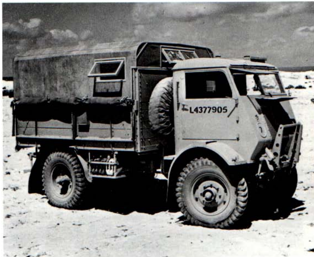
Right: The WOT8 was a shorter wheelbase version of the WOT6, using the same engine and cab, but rated for 30 cwt against 3 tons. Most of the 2516 made were used as gun tractors, but this one was a BBC recording van. It is seen in the Alamein area of the Western Desert, just after delivery in September 1942. (IWM)
