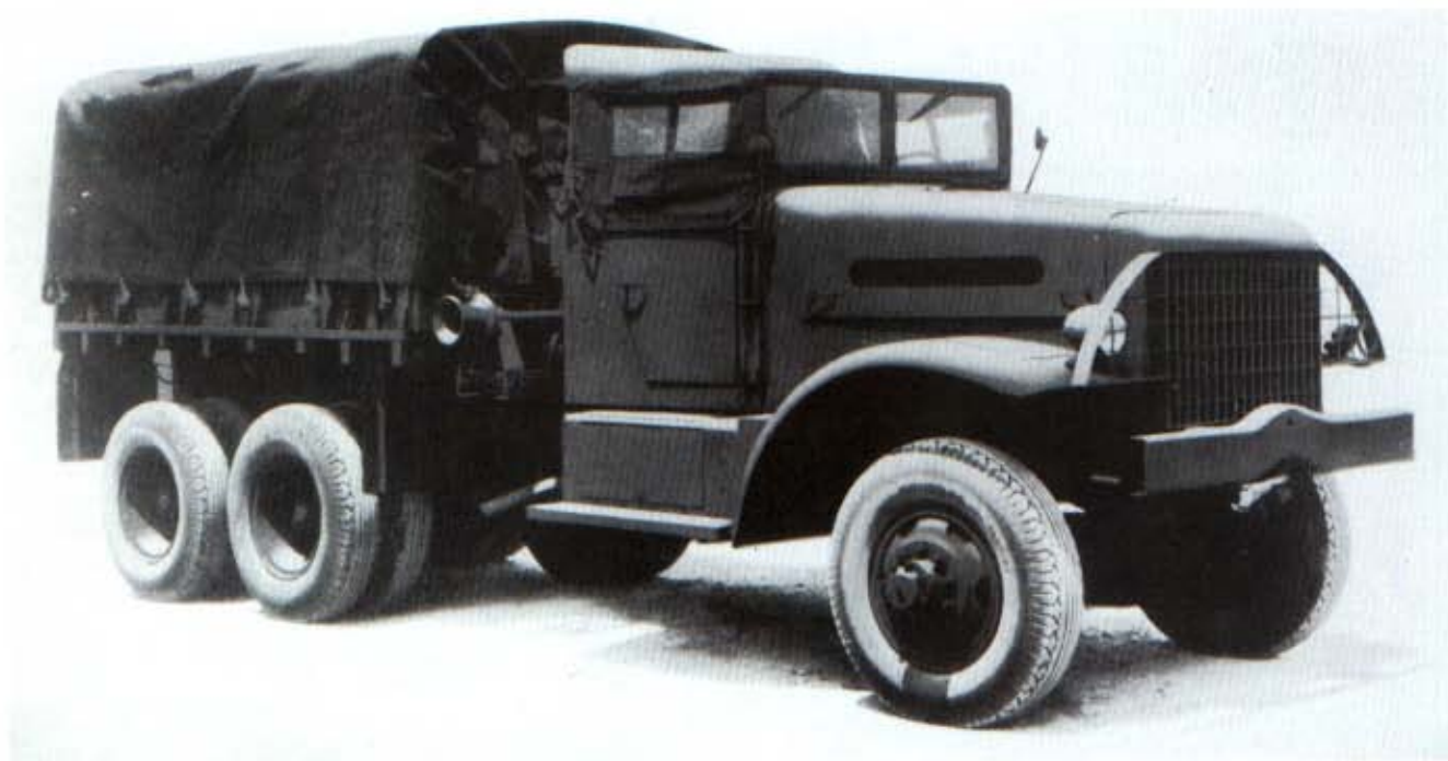
Above: The US Army's standard 6-ton 6x6; this is a Corbitt Model 50SD6 but the same design was made by White, Brockway, Ward La France and FWD. Some Whites and Corbitts had the makers' names on the radiator shell, but most could only be distinguished by the data plate. (Bart Vanderveen Collection)
