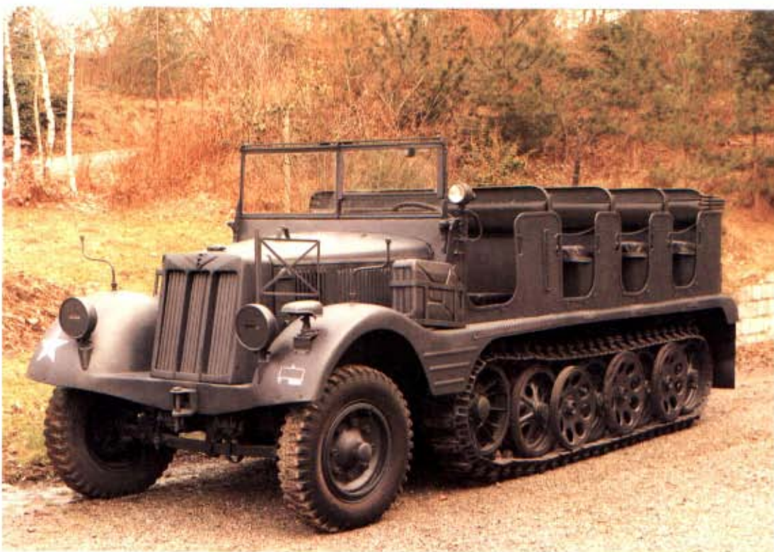
Above: One of the later type of Raupenschlepper-Ost (tracked tractor, east) with open cab, wooden doors and body and Deutz diesel engine. A Steyr design, this example was built by Klockner-Humboldt-Deutz. (Vehicle displayed at the Victory Memorial Museum)
