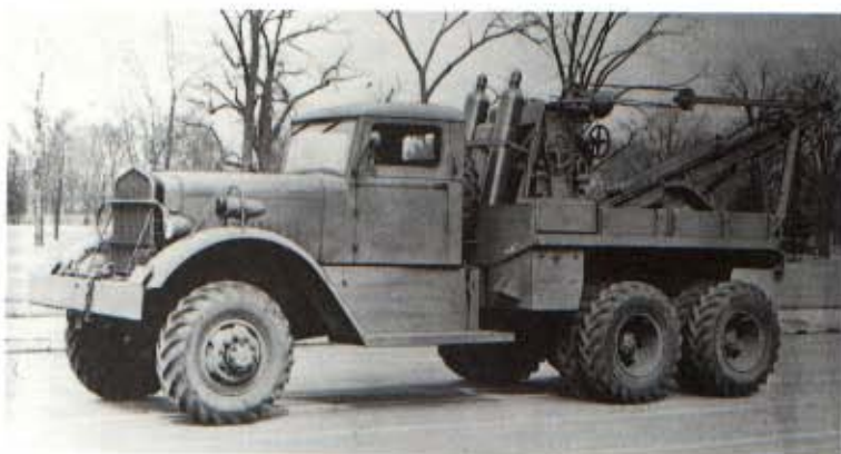
Bottom: C.1941 Ward La France M1 6x6 heavy wrecker with Gar Wood swinging boom crane and front-mounted winch. About 1500 of this design were made by Ward La France and 530 by Kenworth. (Bart Vanderveen Collection)
