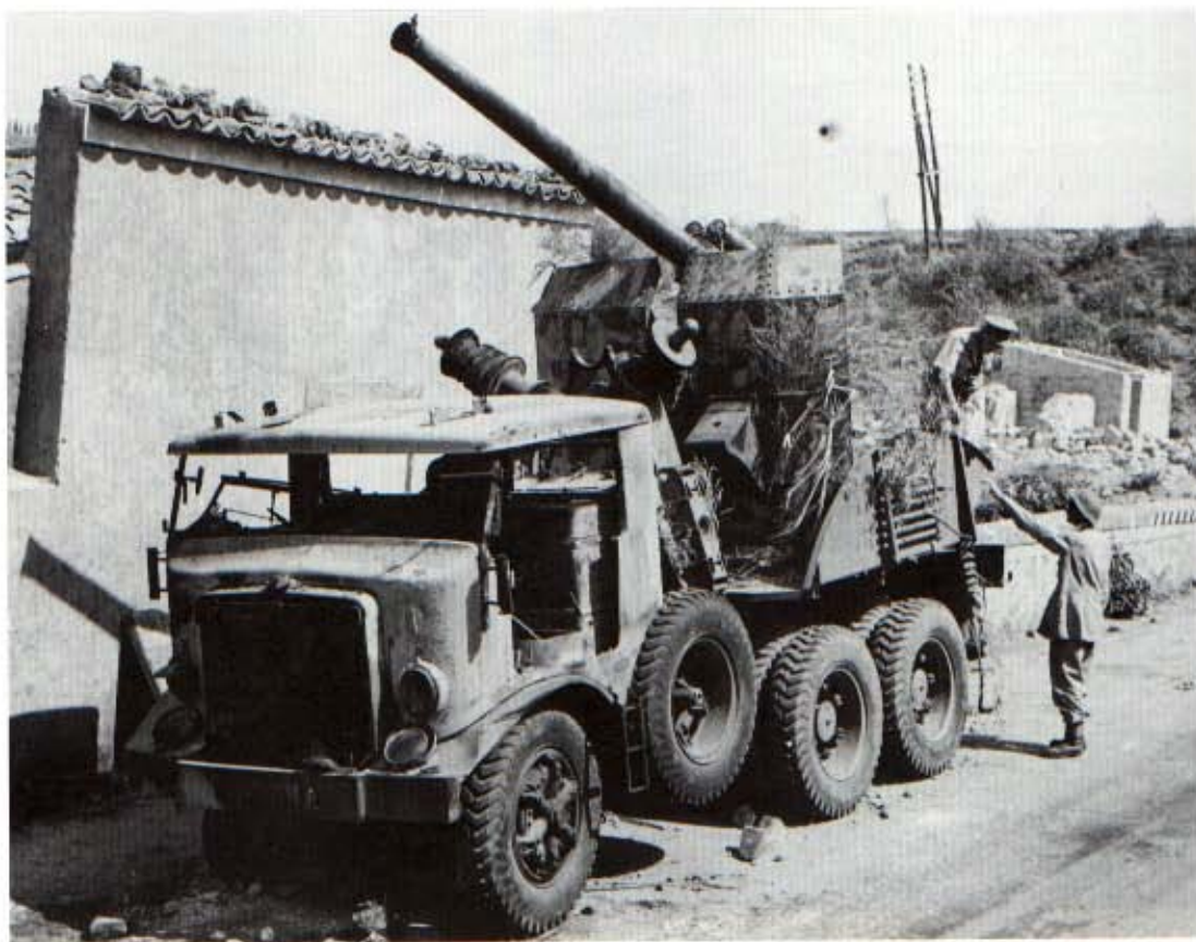
Right: A Breda Tipo 51 heavy 6x4 chassis with Ansaldo 90/55 gun, abandoned near San Michele, Sicily, after the Allied invasion in July 1943. (IWM)
