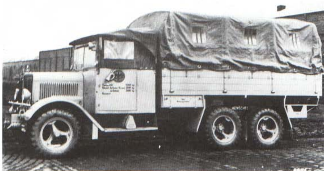
Left: Typical of the 6x4 civilian trucks made during the 1930s and used in large numbers during the war is this Henschel with 10.8-litre 100bhp six-cylinder engine. A wide variety of bodies was built, including signals vans, mobile printing presses, workshops and fire engines. (Nick Baldwin Collection)
