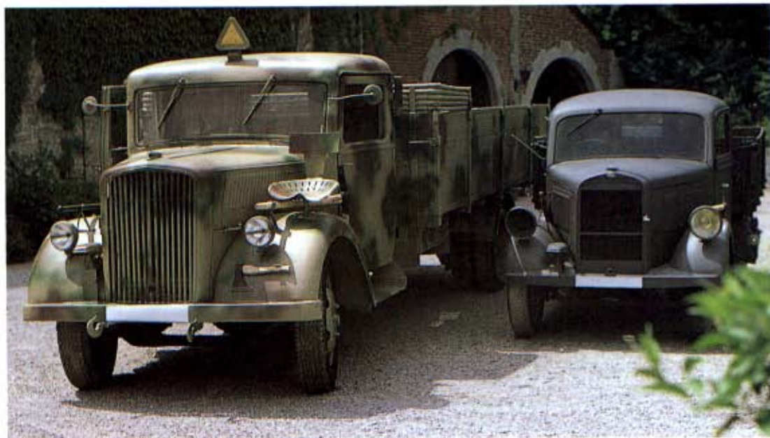
Right: Two Opels, left, a standard 3.5-ton general purpose truck, unusual in having a bus-type cab built by Friedrich Rometsch of Berlin. This company became well-known after the war for cabriolet bodies on Volkswagens. On the right is a smaller Opel, a 1-ton light truck which served as an ambulance with an anti-tank unit. (Vehicles displayed at the Victory Memorial Museum)
