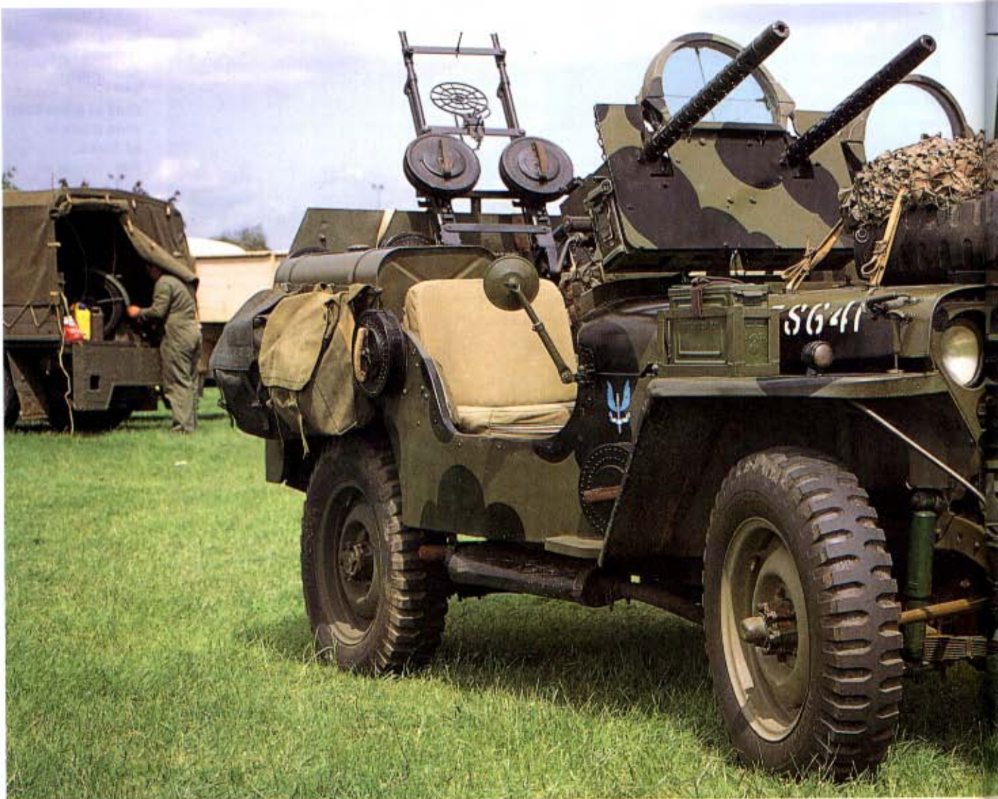
Above: A Willys Jeep with anti-aircraft machine guns front and rear. These were fitted in England for special use by the SAS.
