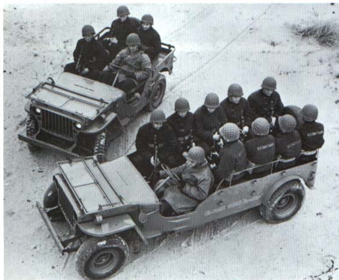
Above: Long wheelbase Jeeps were made in wheeled 6x6 form and as halftracks. They were largely experimental. (The Tank Museum, Bovington)
