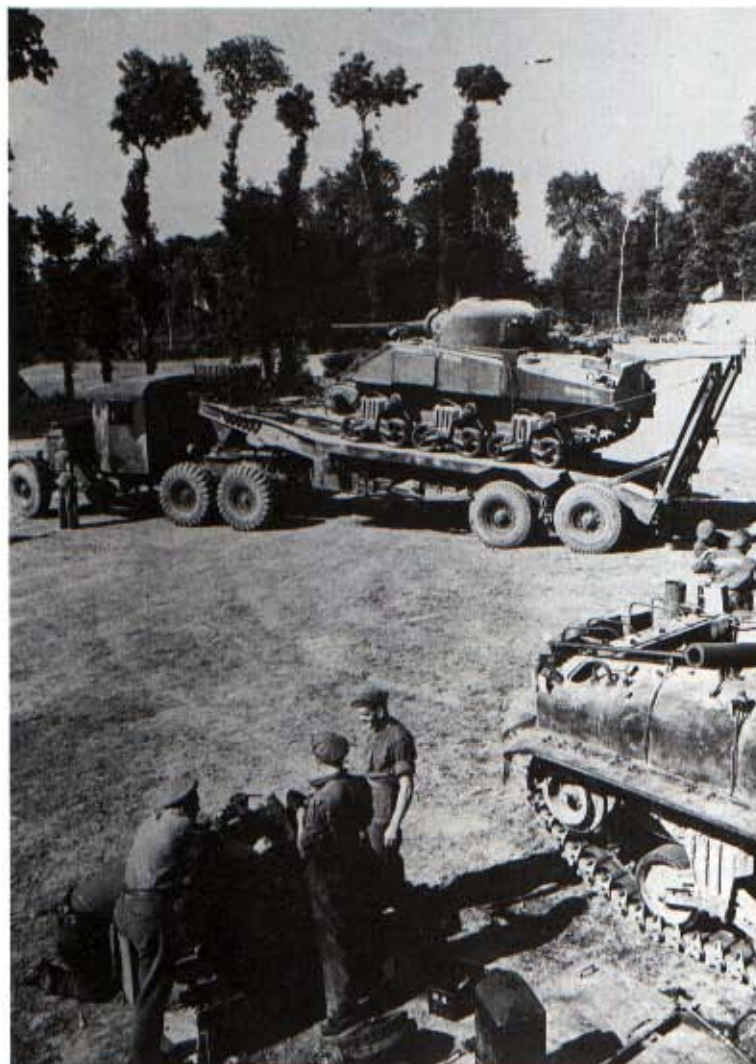
Above: This Scammell Pioneer is bringing a damaged M4 Sherman tank to a REME field workshop in Germany prior to the crossing of the Rhine in early 1945. These workshops moved from one dump of damaged vehicles to another, repairing as many as could be saved. (The Tank Museum, Bovington)
