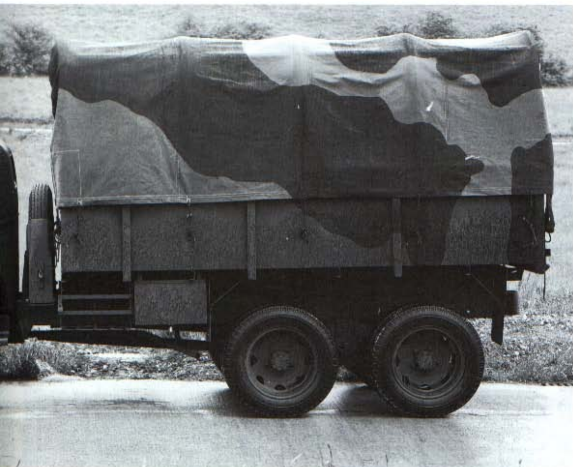
Above: The famous CCKW, 'Deuce and a half' or 'Jimmy', in its standard form. This is a long wheelbase CCKW-353 with enclosed cab. The engine was a 4.4-litre six-cylinder of 94 bhp, driving through a five-speed gearbox with two-speed transfer box and front-axle declutch. There was also a 6x4 of similar appearance, the CCW-353.
