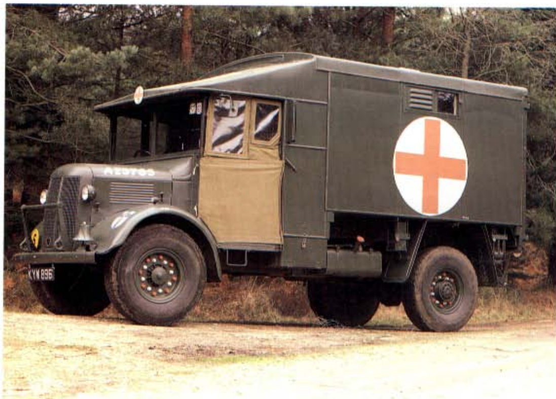
Left: The best known British ambulance of World War Two was the Austin K2, which replaced the other designs from 1940 onwards. More than 13,000 were made. This restored example was discovered in a scrap dealer's yard in Oxfordshire; the owner not only rebuilt it but gradually acquired all the necessary equipment such as stretchers and first aid kit.
