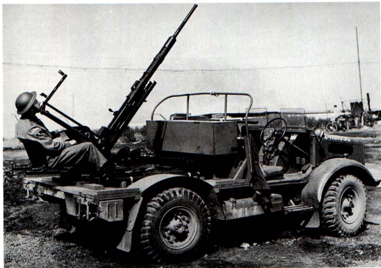
Above: The gun-carrying version of the MW was known as the MWG, but this is an early example on an MWD chassis. It is fitted with a 20mm Polsten anti-aircraft gun. Note the twin aero screens of the early MW models. (NMM)
