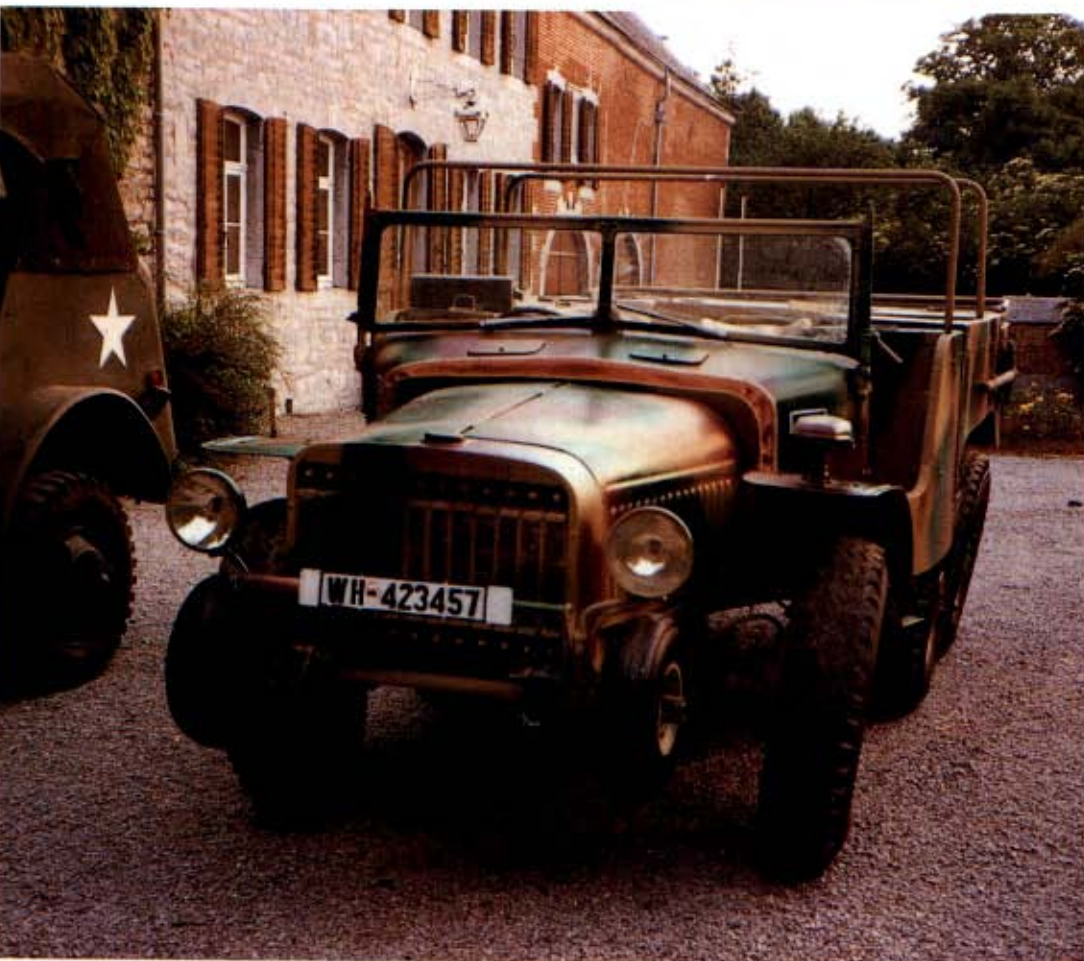
Above: A Latil M2TL6 artillery tractor with four-wheel drive and steering. It has a 3-ton winch and a towing capacity of 5 tons. Made in 1939, it served with the Belgian Army.
