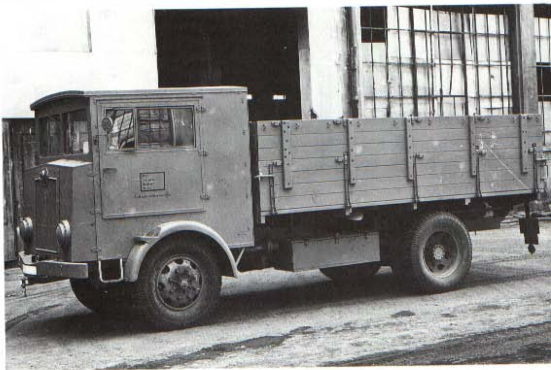
Right: The Fiat 626 had a smaller engine, of 5750cc, in petrol or diesel form, and came in two wheel-bases. This is a 628N built for the German Army in 1942, and has a German-made Einheits military cab. (Fiat Centro Storico/Nick Baldwin Collection)
