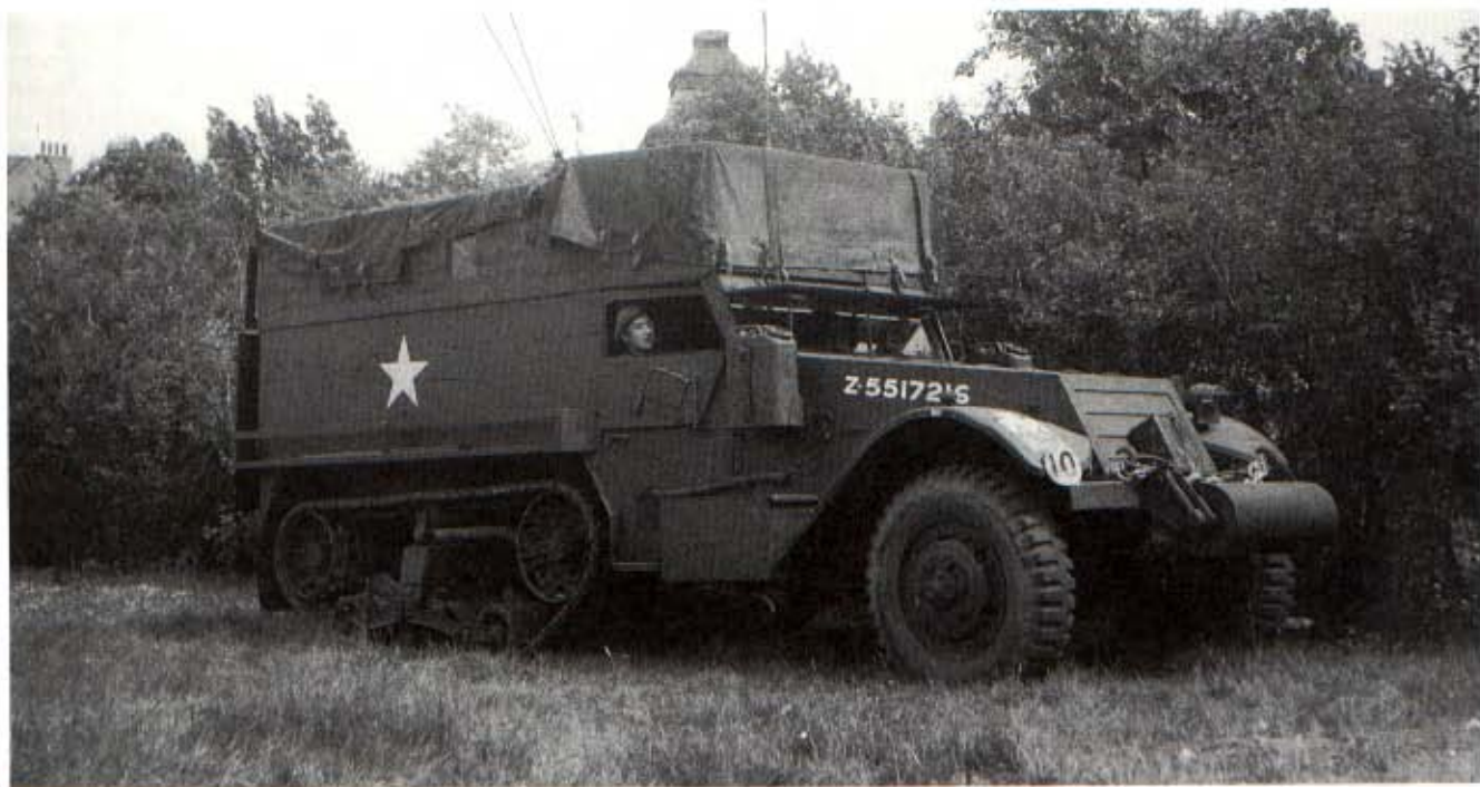
Above: This M series halftrack is being used by the CO of the Field Regimental Section of the Royal Artillery as a wireless vehicle when he was away from HQ. With one wireless working to divisional HQ and the other to the observation posts, it provided a 'step up' or relay to boost the signal over long distances. (IWM)
