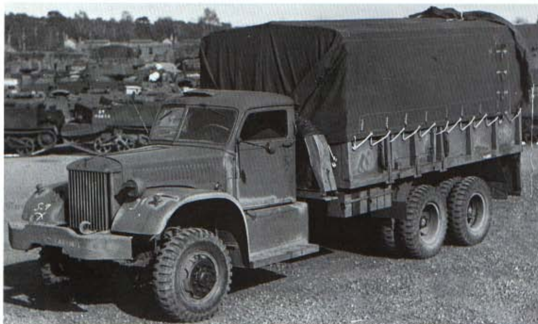
Left: The standard 4-ton 6x6 was made by Diamond T who delivered more than 19,000 for general cargo work as well as wreckers. Standard wheelbases were 151 and 172 inches, but this is a long-wheelbase (201-inch) Model 975A, of which about 1500 were delivered to the Canadian Army. They were fitted with bridging bodies by the Brantford Coach & Body Co of Brantford, Ontario, and used by RCASC bridge companies to transport girders and Bailey bridging equipment, also rafts. The chassis was also used to carry cranes by Bay City and Coles, the latter fitted in England. (Public Archives of Canada)
