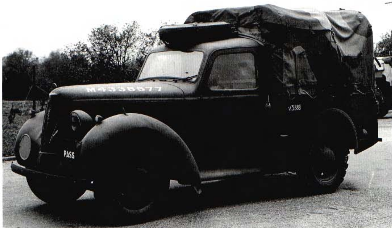
Above: The Hillman light utility was based on the Hillman Minx car. Civilian vans were sold under the name Commer 8cwt, but military versions were all Hillmans. They were made from 1940 to 1945; this is a later version, identified by its wire mesh grille. Earlier ones had civilian type slatted grilles.
