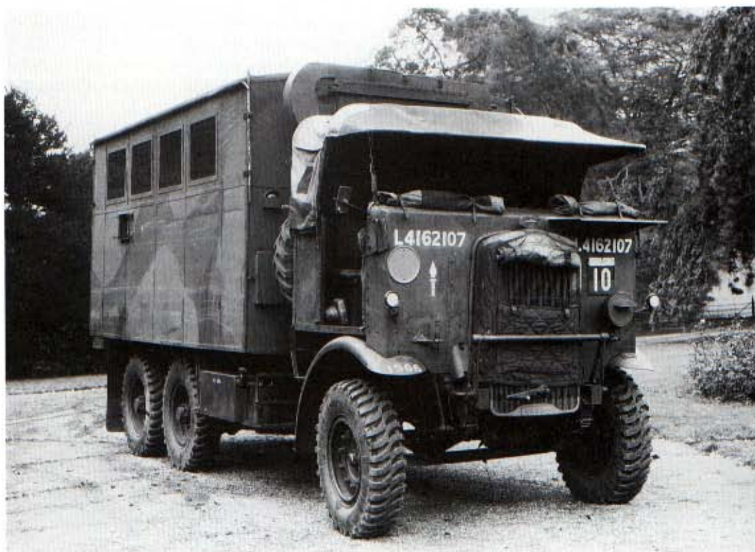
Right: The Leyland Retriever was an older design than the Austin or Fordson, dating back to 1933. This one carries a van body for sound ranging and plotting equipment, used for locating enemy guns. (IWM)
