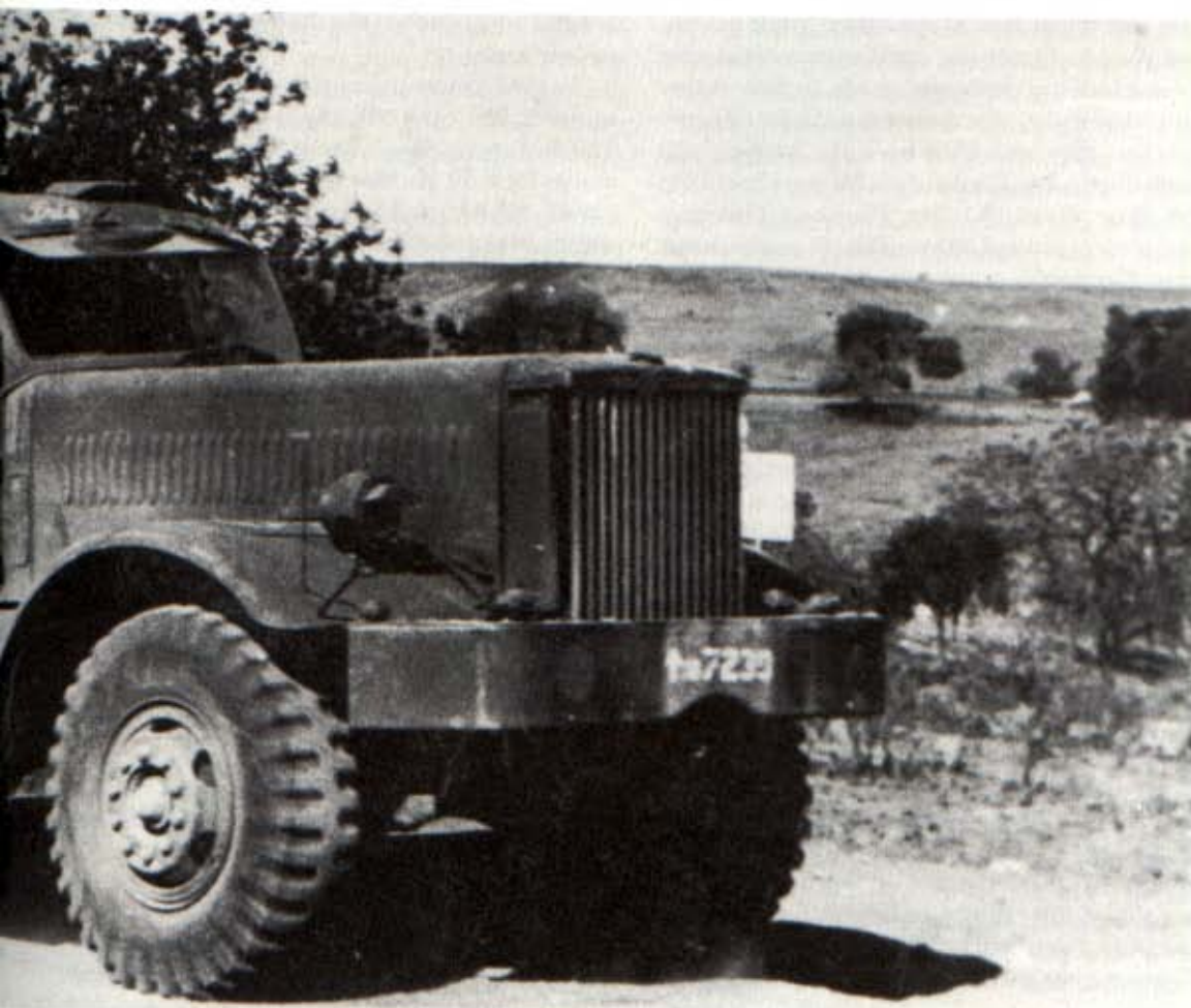
Left: The trailers loaded by the Diamond T 969s were as often as not pulled by Diamond T 980s. These were larger trucks, whose ohv Hercules DXFE diesel engines displaced 14.6 litres. The standard trailer for use with the 980 was the three-axle twelve-wheel M9 for a 45-ton load. This one is carrying a Sherman tank. (The Tank Museum, Bovington)
