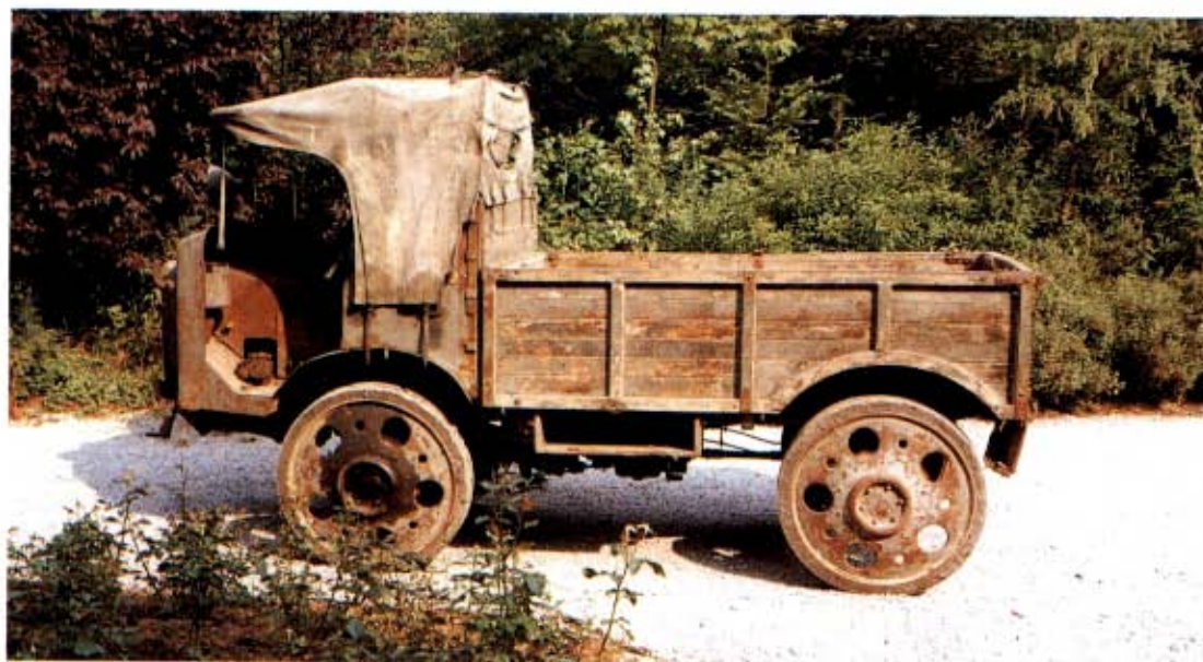
Left: The extraordinary little OM Autocaretta which could be used as a light truck or artillery tractor. It was powered by a 1616cc air-cooled engine, and drove and steered on all four wheels. Most had solid tyres, as here, though pneumatics could be fitted. It was made from 1933 until about 1944. (Vehicle displayed at the Victory Memorial Museum)
