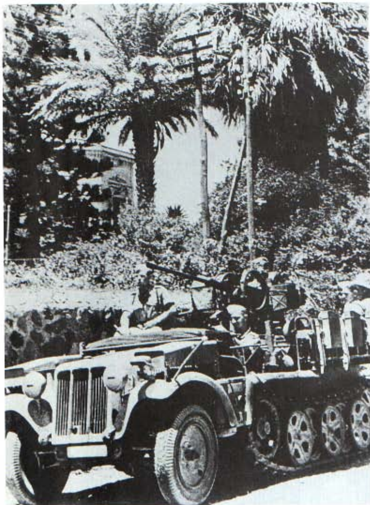
Above: Apart from the Kettenkrad, the smallest half-track tractor was the Demag D7 (Sd.Kfz.10), rated as a 1-tonner. Powered by a 4.2-litre six-cylinder Maybach engine, it had a preselector gearbox with seven forward speeds and three reverse. Maximum speed on roads was about 40mph. This example is carrying a light anti-aircraft gun. (IWM)
