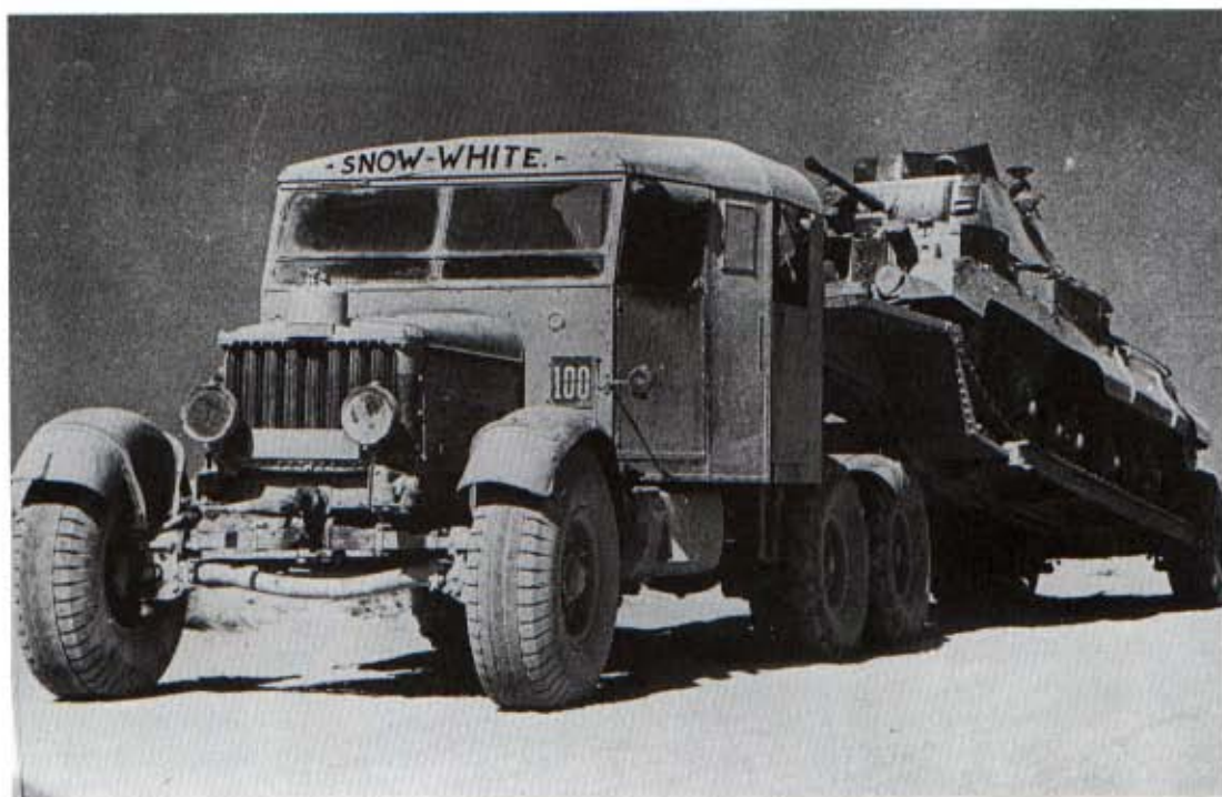
Above: This Scammell Pioneer is bringing a damaged M4 Sherman tank to a REME field workshop in Germany prior to the crossing of the Rhine in early 1945. These workshops moved from one dump of damaged vehicles to another, repairing as many as could be saved. (The Tank Museum, Bovington)
