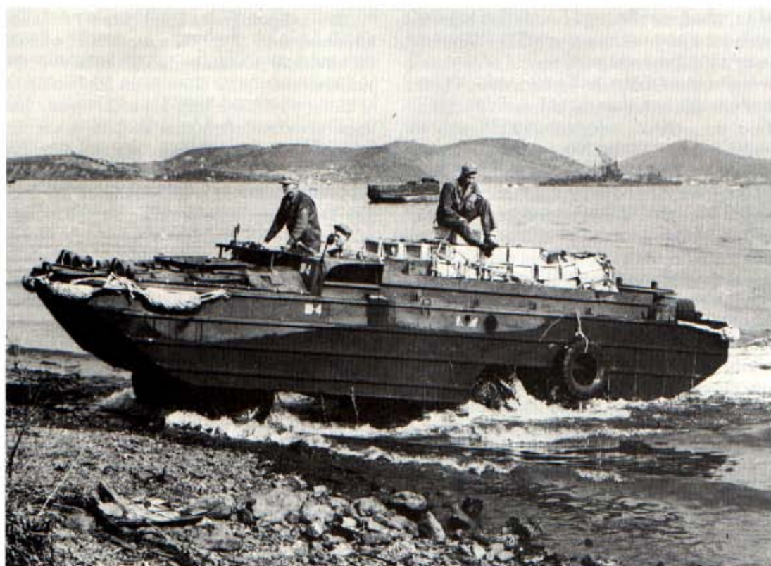
Above and left: Two examples of the GMC DUKW 6x6 amphibian, during the landing at Hollandia, New Guinea in 1943. The crane for loading/unloading was a necessity as the DUKW had no ramp, a deficiency put right by the Russians with their version on the ZIL-151 chassis. (VWM)
