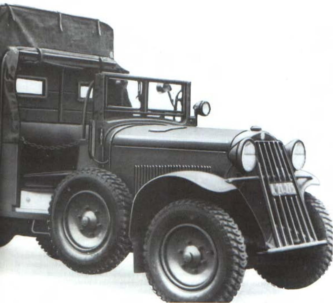
Left: The Austrian-built Steyr 640 was a 1½-ton 6x4 truck. Of the 3780 made between 1937 and 1941, nearly all went to the Wehrmacht. This is the standard truck version, but it was also used as a command car and ambulance. The spare wheels were mounted behind the front axle, and served as belly supports when the truck was negotiating rough ground.
