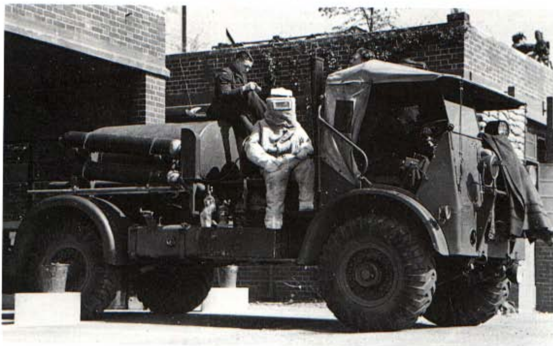
Left: The Crossley Q-type 4x4 was made in several forms, including a GS truck/mobile workshop and fire tender on the longer wheelbase, and a tractor for semi-trailers or full trailers. This is a fire tender for the RAF. (The Tank Museum, Bovington)
