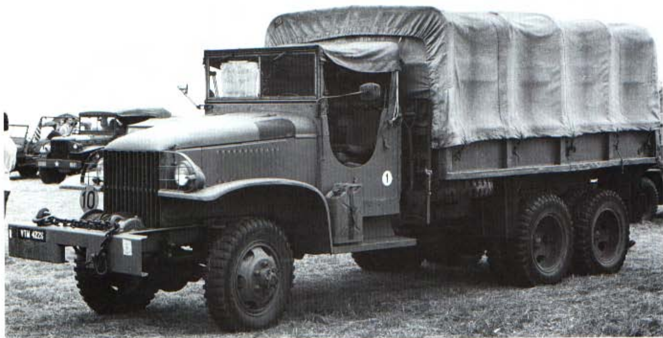
Above: A CCKW-353 with canvas-topped cab and cut-away doors. It is fitted with a winch which was optional on all CCKWs.
