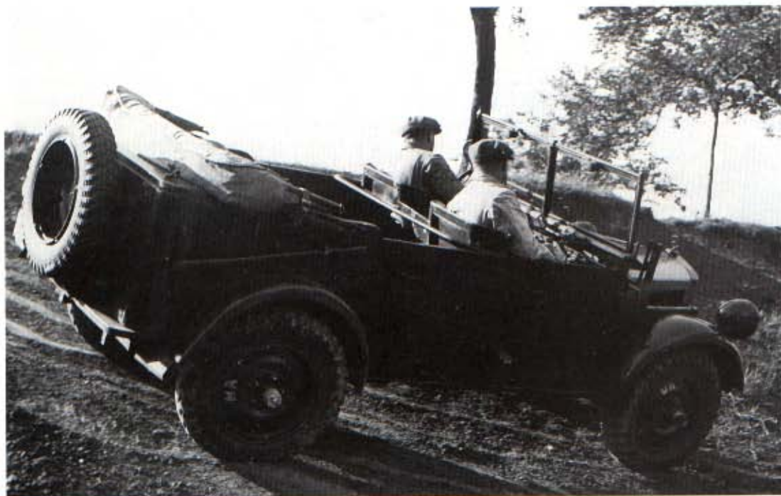
Left and Below: Mercedes-Benz contribution to the light cross-country vehicle programme was the G5, powered by the company's 2-litre side-valve engine. It was less powerful than the ohv Stoewer of the same size. It was not ordered by the Wehrmacht in large numbers; only 300 were made between 1937 and 1941. Some were used by the Hungarian Army after the war. (NMM)
