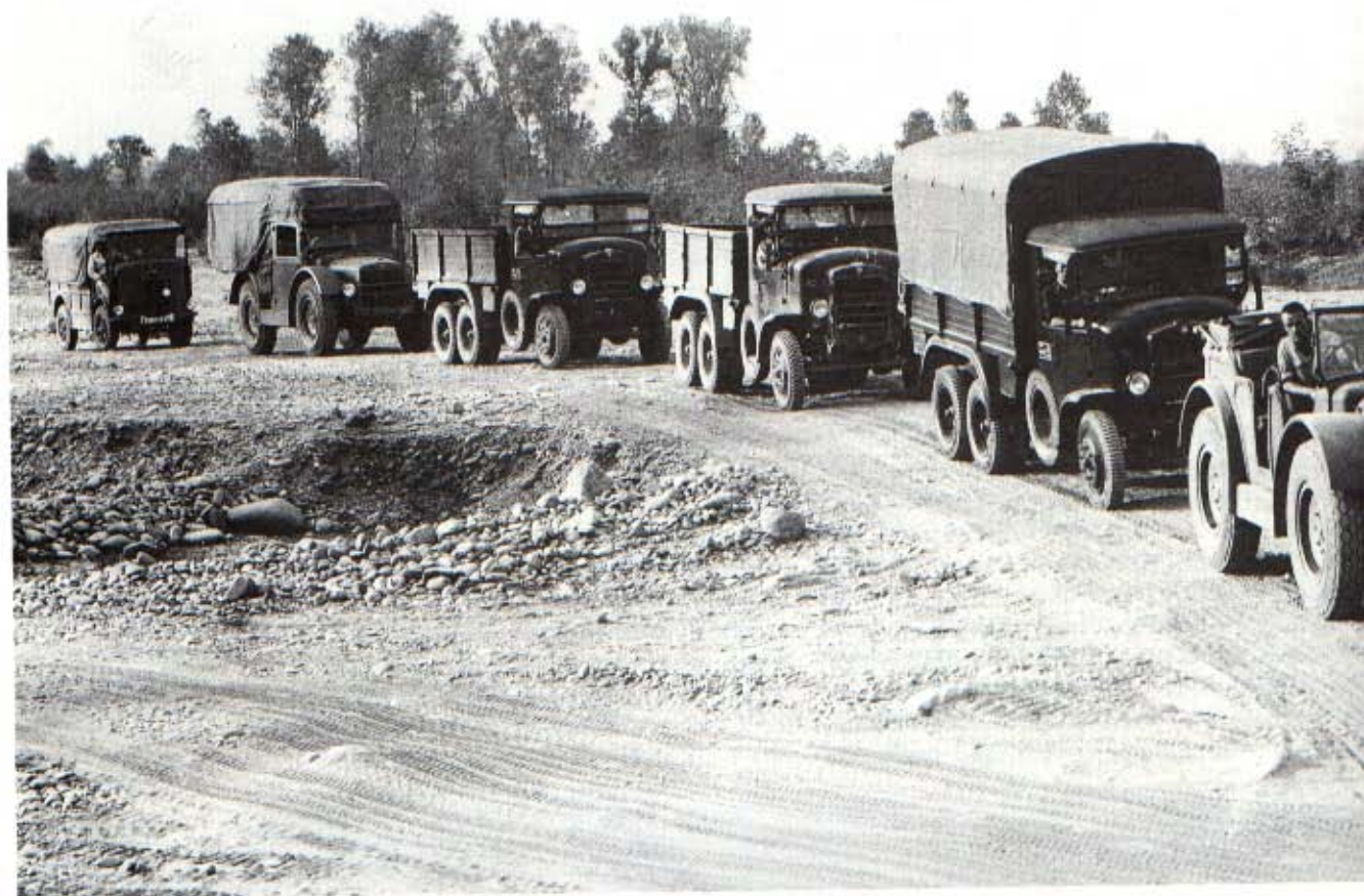
Right: The Fiat 626 had a smaller engine, of 5750cc, in petrol or diesel form, and came in two wheel-bases. This is a 628N built for the German Army in 1942, and has a German-made Einheits military cab. (Fiat Centro Storico/Nick Baldwin Collection)
