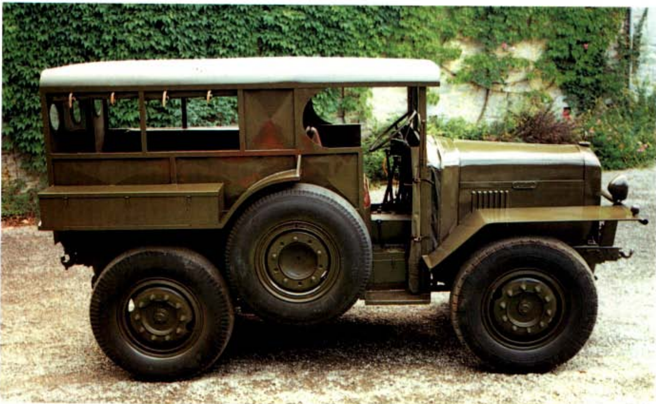
Above: A Latil M2TL6 artillery tractor with four-wheel drive and steering. It has a 3-ton winch and a towing capacity of 5 tons. Made in 1939, it served with the Belgian Army.
