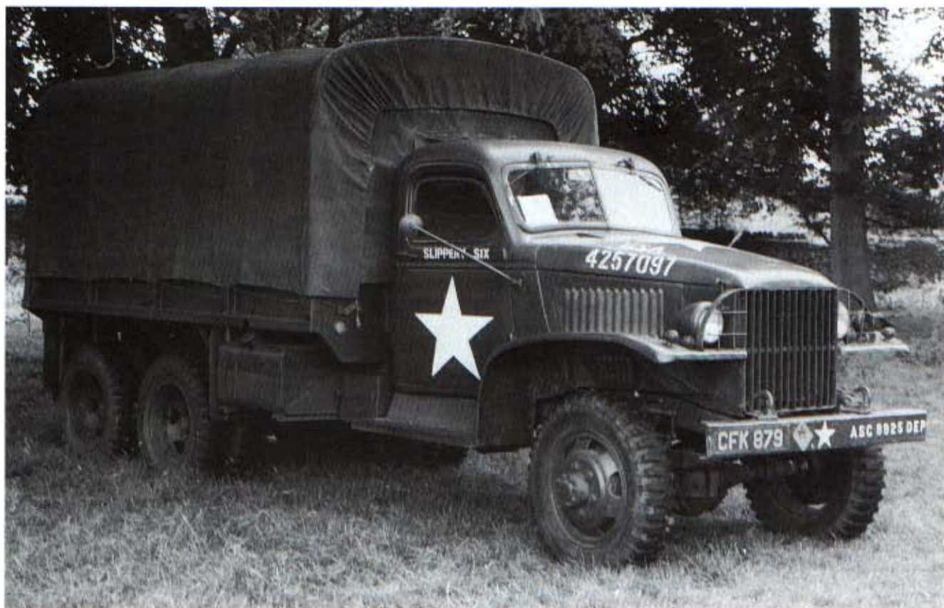
Above: The famous CCKW, 'Deuce and a half' or 'Jimmy', in its standard form. This is a long wheelbase CCKW-353 with enclosed cab. The engine was a 4.4-litre six-cylinder of 94 bhp, driving through a five-speed gearbox with two-speed transfer box and front-axle declutch. There was also a 6x4 of similar appearance, the CCW-353.
