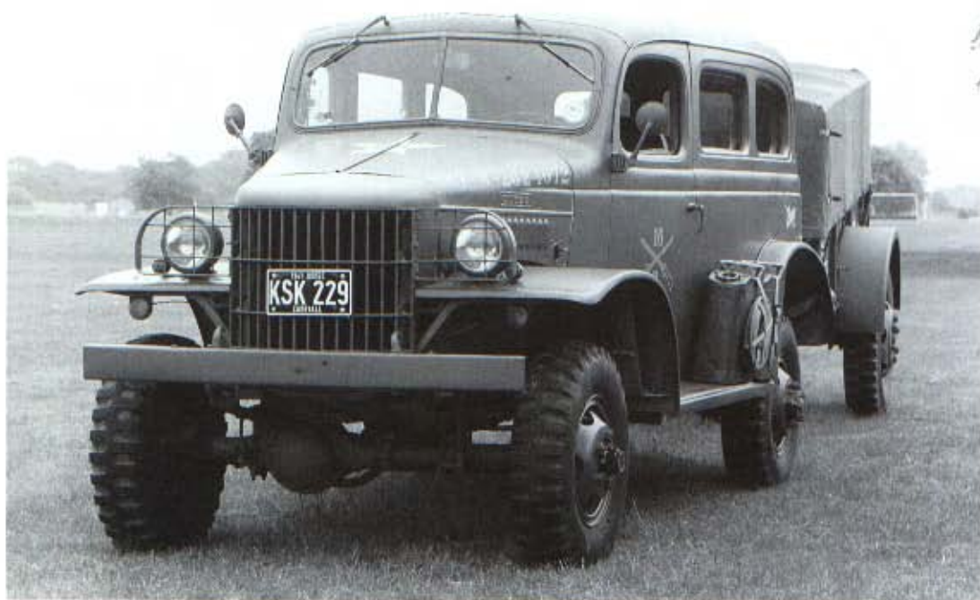
Left: The Dodge WC17 Carryall was a hybrid vehicle, using the body of the civilian Suburban with militarised front end and bonnet. It was rated for 1½ ton loads, and in 1942 gave way to the lower and wider T 214 which was rated as a ¾ tonner. (The Tank Museum, Bovington)
