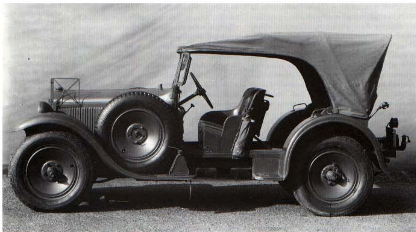
Below: An early 1930s Kübelwagen on the Mercedes-Benz 260 chassis, with body by Gaubschat. Later versions had doors. (Daimler-Benz)
