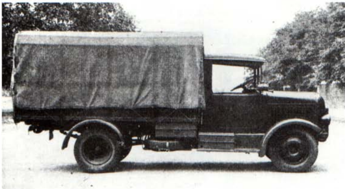
Left: An older design of medium 4x2 truck was the SPA 36/38 with 4-litre petrol engine, introduced in 1936. This is a standard G5 truck, but the chassis also carried workshop, ambulance and bus bodies. (Bart Vanderveen Collection)
