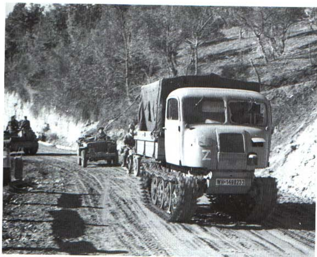
Left: A Raupenschlepper Ost (tracked tractor, East) in its closed cab version with Steyr air-cooled V8 engine. Steyr built 2600, Graf und Stift about 4500 and Auto Union 5600. The rest came from the Klockner-Humbolt-Deutz (Magirus-Deutz) factory, which also supplied engines for the later RSO/03. This one was captured by British troops in Italy, and is seen at Fossacesia, south-east of Pescara, taking supplies to the front line. (IWM)
