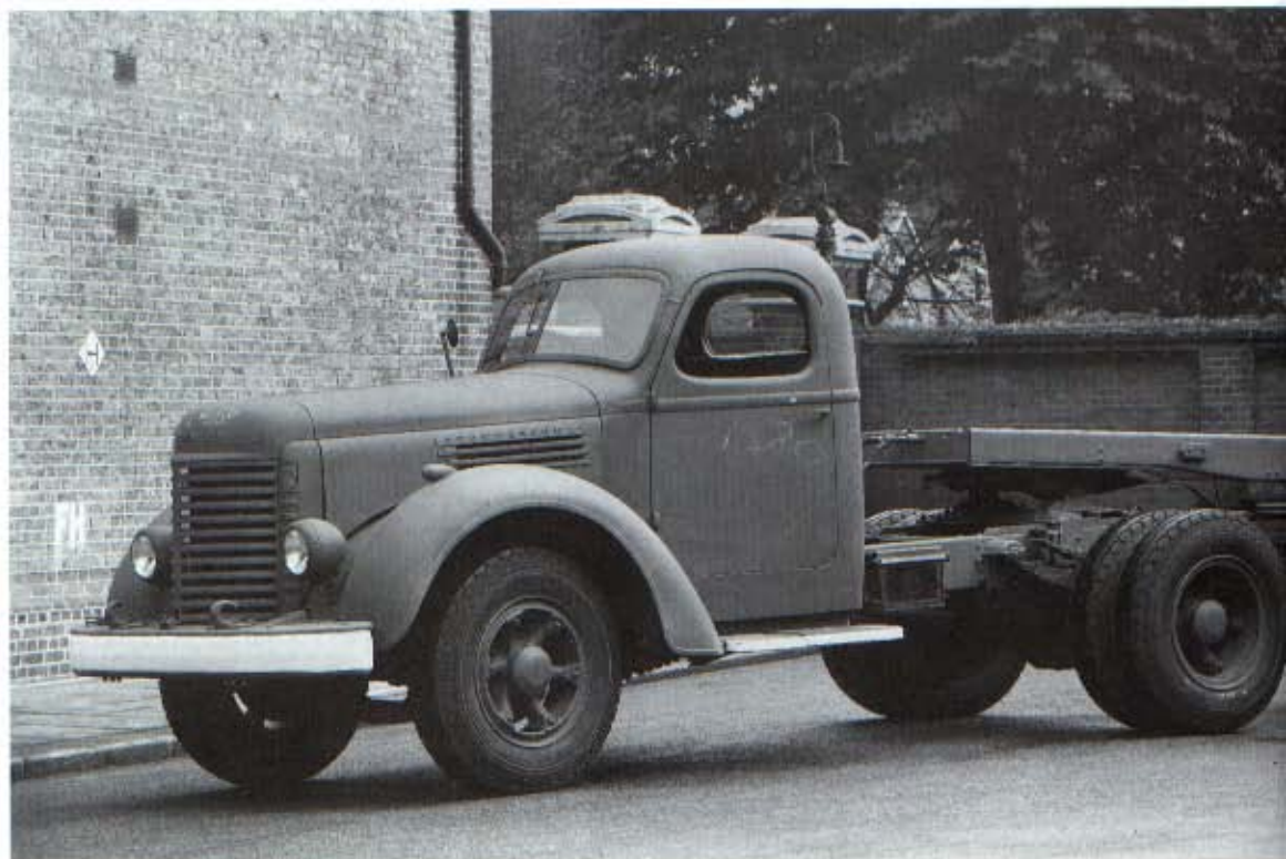
Right: The first Internationals supplied to the US Army in 1940 were of the newly introduced K line. This is a KR8 tractor on a 137-inch wheelbase, coupled to a Fruehauf 10-ton semi-trailer. (NMM)
