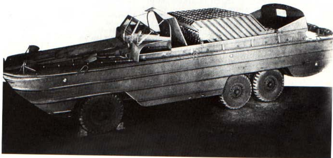
An experimental DUKW, the Scorpion, fitted with a 4.5mm rocket launcher which could fire 120 rounds in a few seconds.
