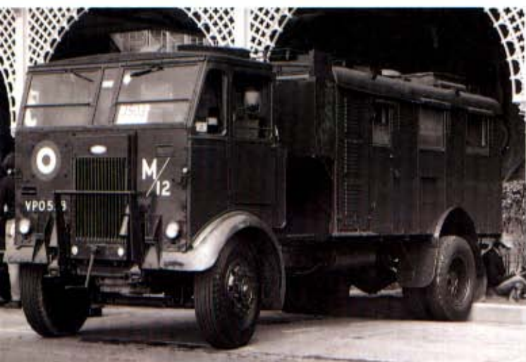
Top: The Leyland Hippo II 10-ton 6x4 was introduced in 1944 and was distinguished from the Hippo 1 by its closed cab and more powerful, though smaller, engine. (Peter Daniels/NMM)
