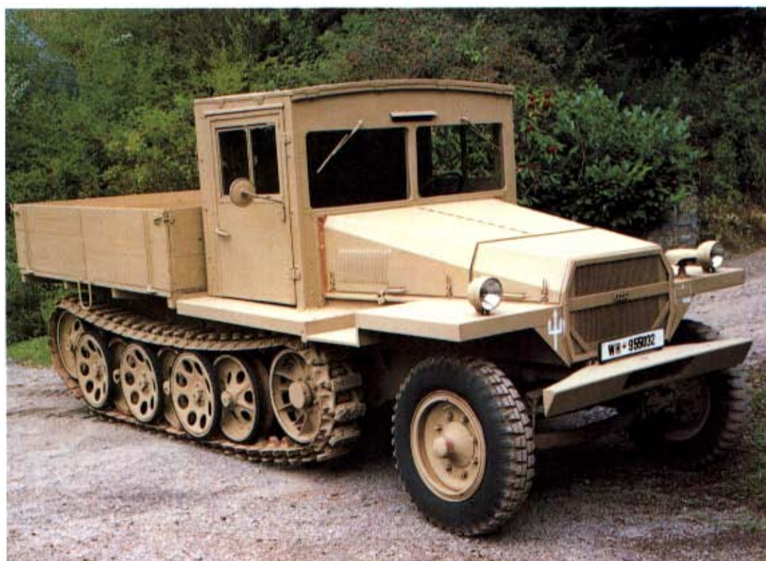
Above: The lightest of the German halftracks was the Sd.Kfz 10 for towing a 1 ton load. Designed and developed by Demag as the D7, it was also made by Adler, Büssing-NAG, MIAG, Phänomen and Saurer.
