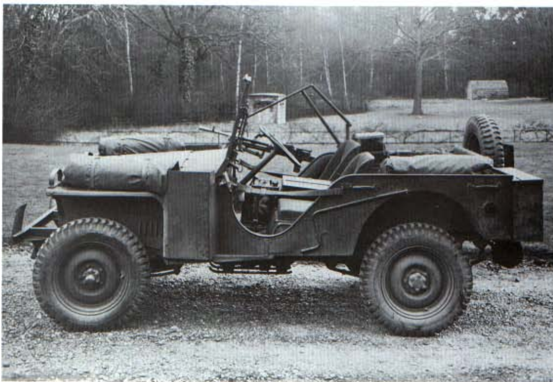
Above and left: One of the 1642 Bantam-built BRC Jeeps, fitted with a Browning M2 machine gun. (The Tank Museum, Bovington)
