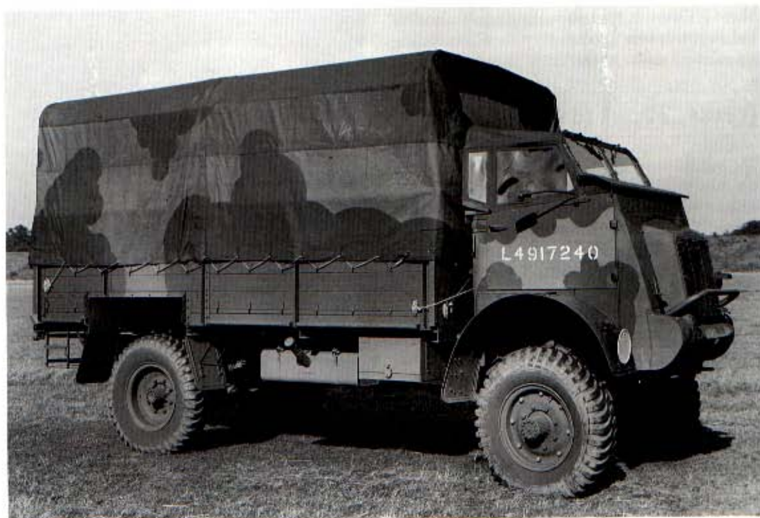
Right: The only QL to be produced with a soft-top cab was a special QLC designed to carry a 6 pound anti-tank gun. They were intended for desert use, and when the North African campaign was completed, they were reworked and fitted with GS bodies, as here. (NMM)
