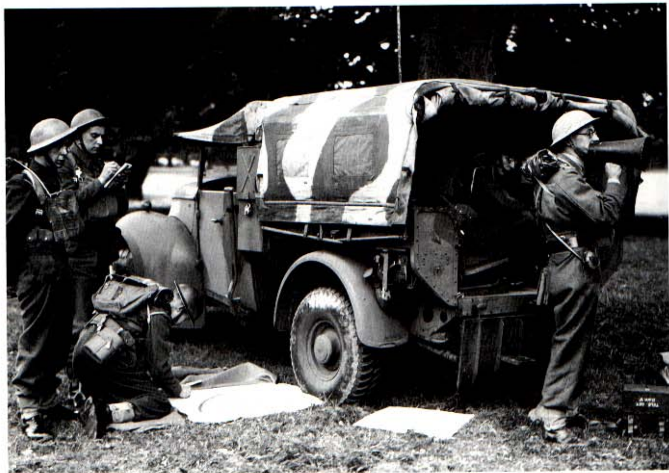
Above. More powerful than the British 'Tillies' was the Ford WOC1, an Anglo-American design using the chassis of the American Ford V8 light commercial with British-built open-cab bodies made by Briggs. Just 2000 were built between December 1939 and July 1940, when the WOC1 was dropped in favour of the 15cwt WOT2. This one is at a Battery Command Post during combined manoeuvres of the Royal Artillery and King's Shropshire Light Infantry. (IWM)
