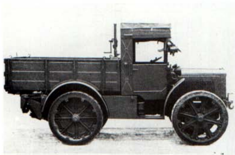
Above: A Breda Trattore Pesante (Heavy Tractor) Tipo 32, powered by the company's own 8136cc four-cylinder petrol engine, and having a five-speed gearbox and four-wheel drive. It was built from 1932 to about 1939, when some were updated with pneumatic tyres and a diesel engine. Its successor was the Tipo 40. (Bart Vanderveen Collection)
