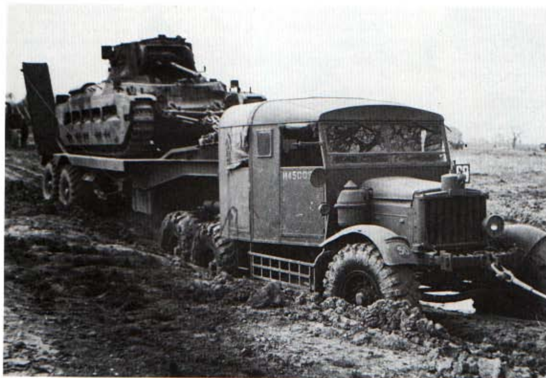
Left: The Pioneer had a reputation for getting out of almost any tight spot, and of rescuing other vehicles as well. It is carrying a Matilda tank on its 30-ton trailer. (The Tank Museum, Bovington)
