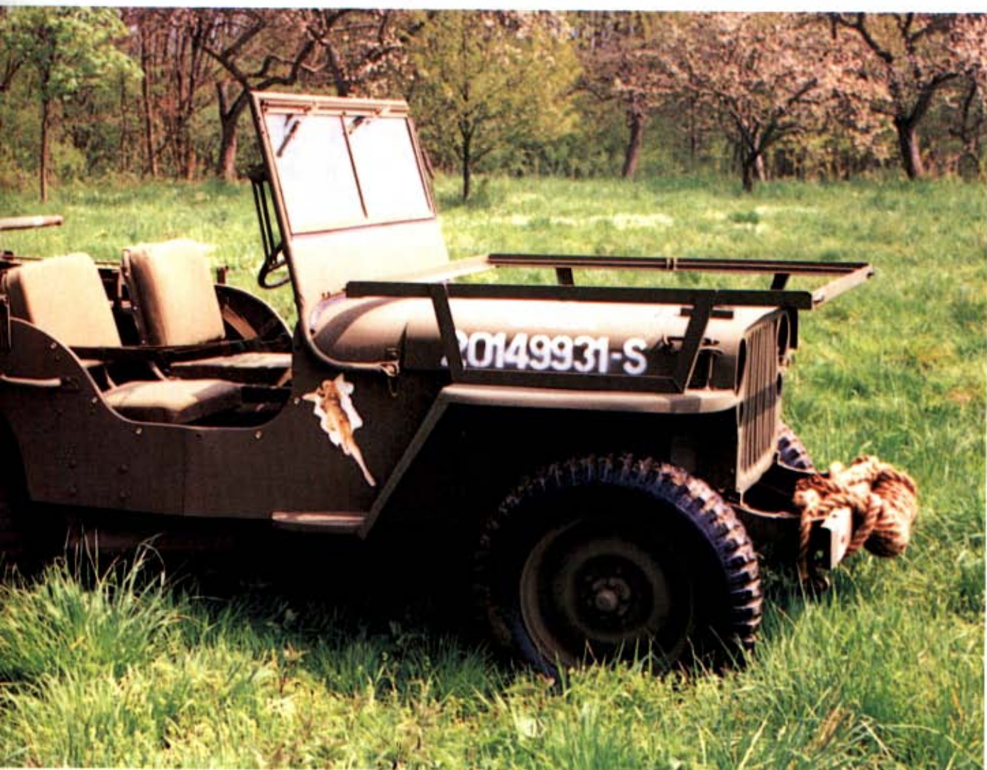
Below: A Jeep transformed into an ambulance, with two stretchers over the bonnet and two at the rear. It was operated by 633 Medical Battalion, First Army. (Vehicle displayed at the Victory Memorial Museum)
