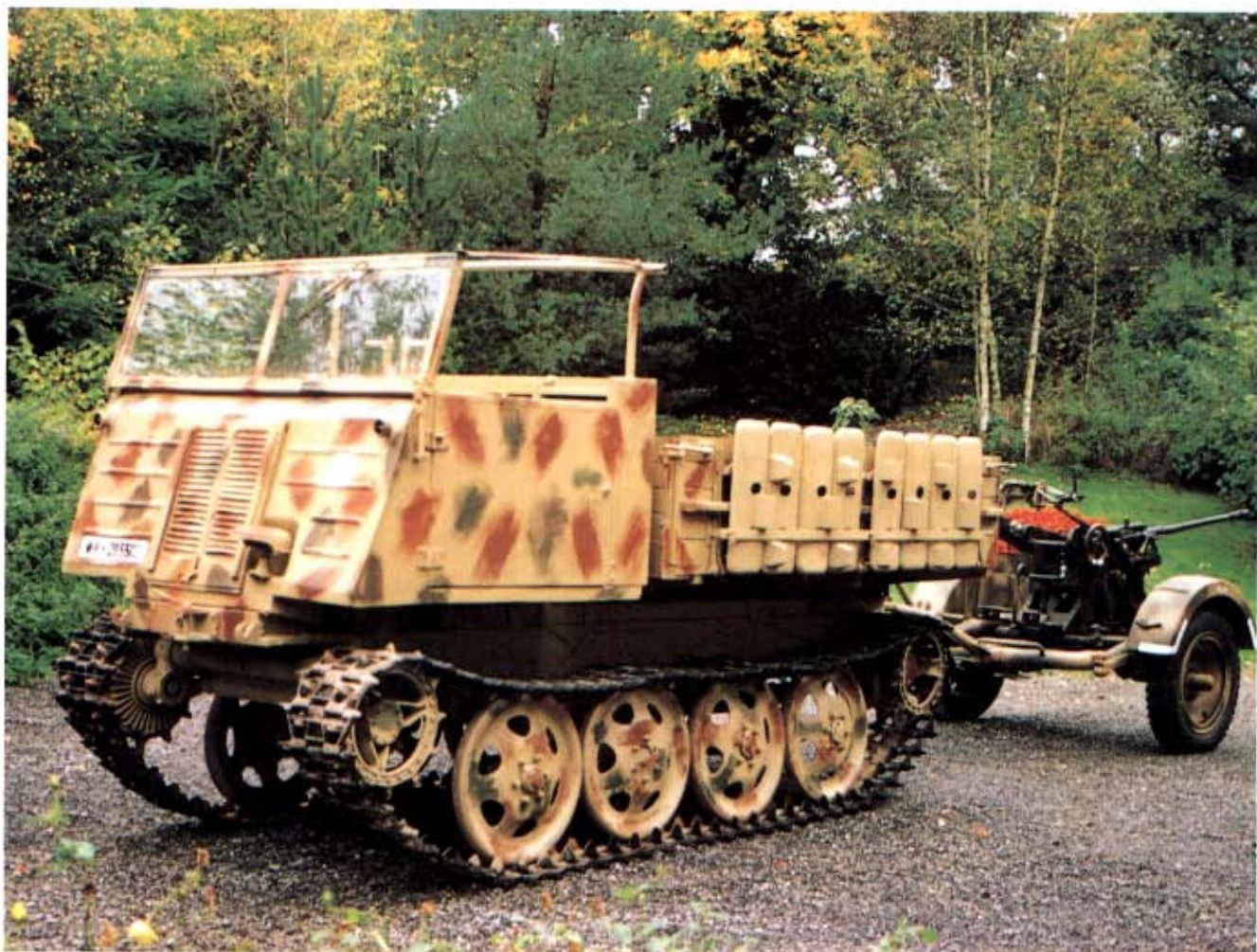
Above: One of the later type of Raupenschlepper-Ost (tracked tractor, east) with open cab, wooden doors and body and Deutz diesel engine. A Steyr design, this example was built by Klockner-Humboldt-Deutz. (Vehicle displayed at the Victory Memorial Museum)
