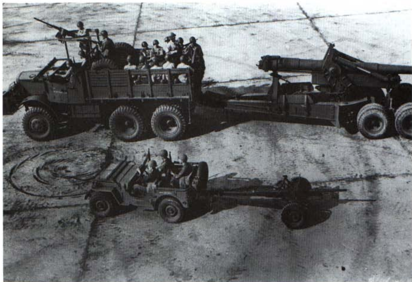
Above: A Mack NO towing a 155mm gun. Above the open cab is a machine gun; every fourth NO made was fitted with an M36 ring mount to take a .30 or .50 calibre machine gun. Contrasted with the Mack is a Jeep towing an anti-tank gun.
