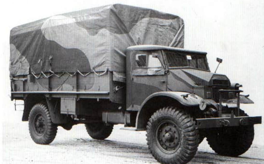
Right: Ford F60L with early type cab (1941) and British-built 3-ton GS body.
