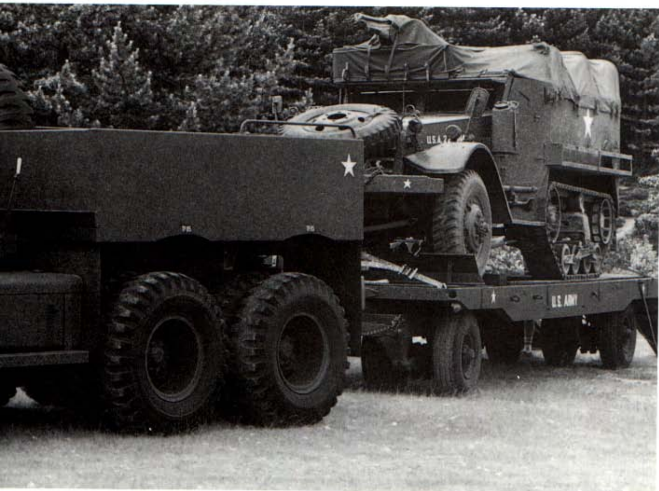
Above: A restored Diamond T 980 towing a two-axle trailer carrying an M series halftrack. (The Tank Museum, Bovington)
