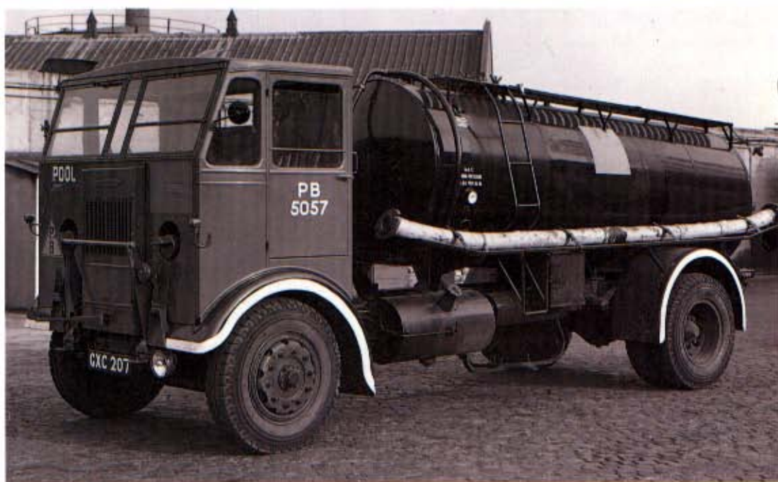
Top: The Leyland Hippo II 10-ton 6x4 was introduced in 1944 and was distinguished from the Hippo 1 by its closed cab and more powerful, though smaller, engine. (Peter Daniels/NMM)
