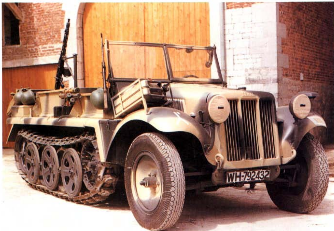
Above: The lightest of the German halftracks was the Sd.Kfz 10 for towing a 1 ton load. Designed and developed by Demag as the D7, it was also made by Adler, Büssing-NAG, MIAG, Phänomen and Saurer.
