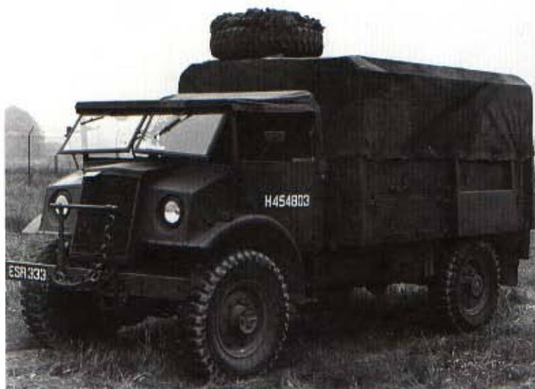
Above: This Ford-built CMP 3-ton truck is a F60S (F=Ford, 60cwt S=short wheelbase). The wheelbase was 134inches, compared with 158inches for the F60L.
