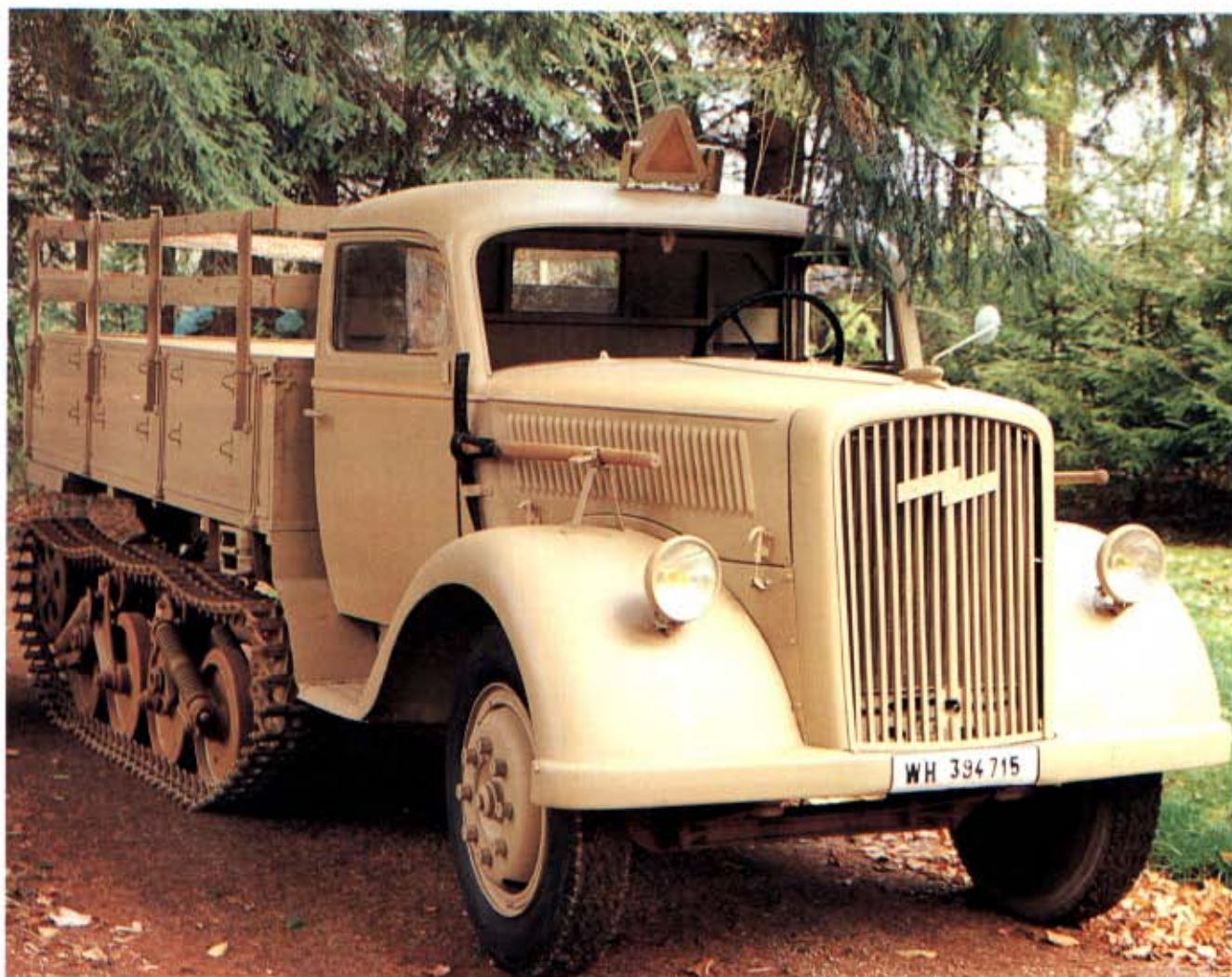
Below: One of several types of halftrack truck was this Opel 2 tonner. It used the standard 3.5-litre six-cylinder engine driving the front sprockets through a five-speed gearbox. (Vehicle displayed at the Victory Memorial Museum)
