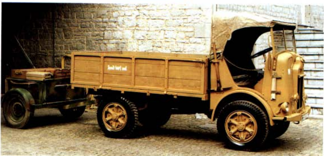
Centre: The SPA CL39 was a light 4x2 truck for infantry support. Its engine was a surprisingly small four-cylinder unit of 1628cc. A variant was the CLF39 which had 700-18 solid tyres, while this example has 210-18 pneumatics. (Vehicle displayed at the Victory Memorial Museum)
