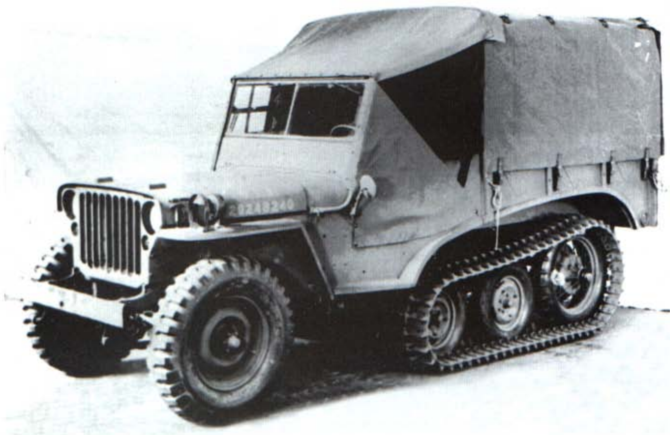
Above: Long wheelbase Jeeps were made in wheeled 6x6 form and as halftracks. They were largely experimental. (The Tank Museum, Bovington)
