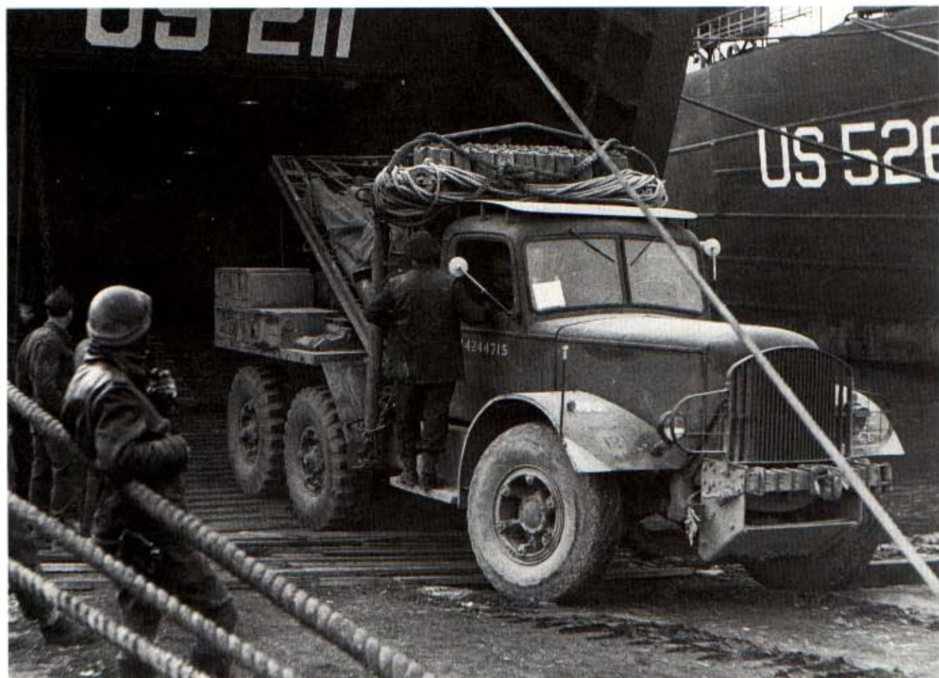
Below: A Mack LMSW 6x4 heavy wrecker with body equipment by Gar Wood. This included an oxy-acetylene welding and cutting gear. It is emerging from a landing craft, probably on the Normandy beachhead in 1944. (Public Archives of Canada)
