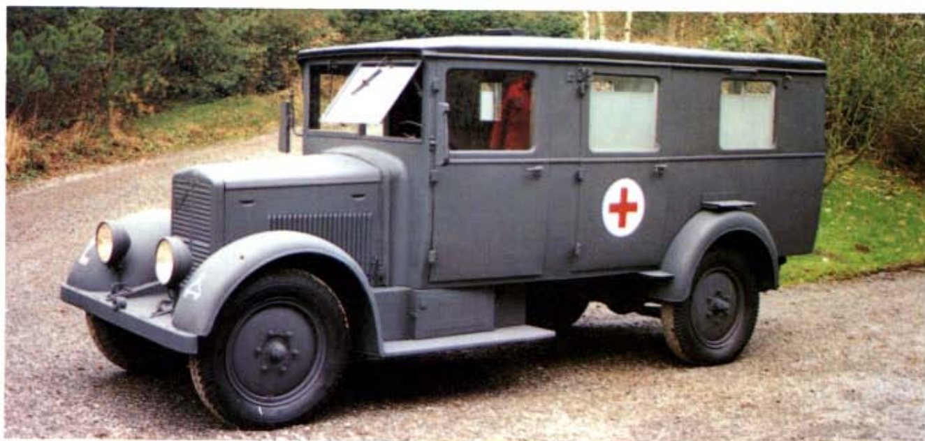
Below: A Phänomen Granit Type 25H of the 3rd Panzer Division. These air-cooled vehicles were among the most popular ambulances in use by the Wehrmacht. (Vehicle displayed at the Victory Memorial Museum)
