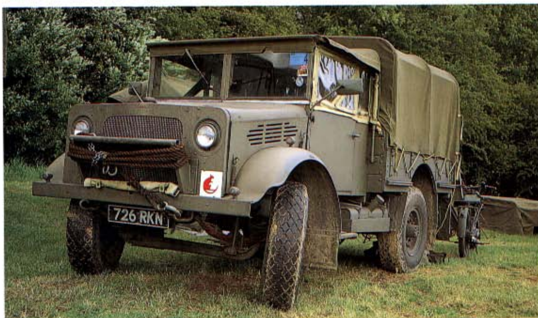
Right: A standard Bedford MWD 15cwt truck. Nearly 66,000 MWs were made in many different versions.
