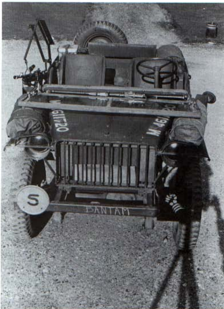
Above and left: One of the 1642 Bantam-built BRC Jeeps, fitted with a Browning M2 machine gun. (The Tank Museum, Bovington)
