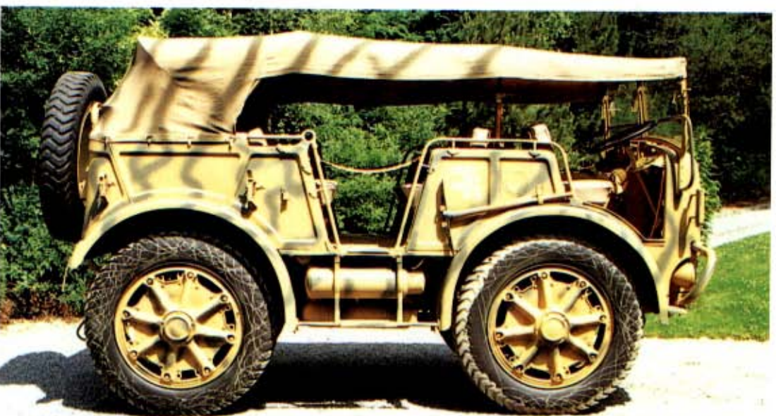
Left: Fiat's 4x4 medium artillery tractor was made in the SPA factory and known as the TM40. Also available with solid tyres, it was powered by a 9365cc 110bhp six-cylinder engine. It was also made in truck form (T40) with German Einheits cab. (Vehicle displayed at the Victory Memorial Museum)
