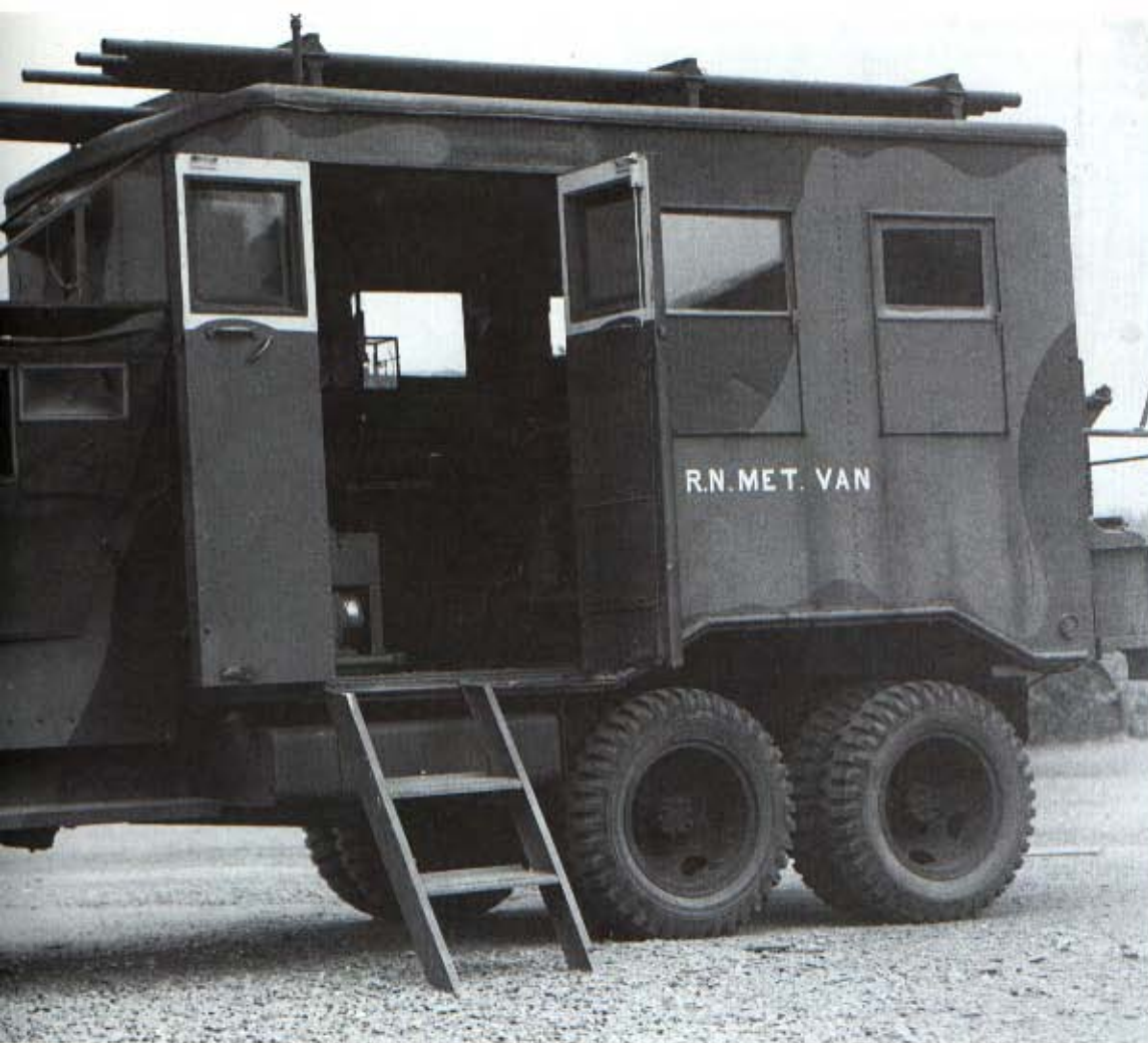
Left: More than 20 types of van body were built on the CCKW, including mobile command posts and workshops. This is a meteorological van for the vitally important task of weather forecasting at the time of the D-Day landings. Completely self-contained, it was equipped for receiving and transmitting information by radio. Only one was made. (NMM)
