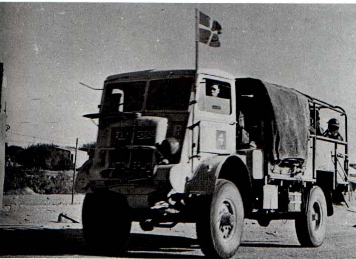
Left: A QLC belonging to an Armoured Division enters Sirte, Libya, in early 1943, after it had been abandoned by Axis troops. To eliminate glare the windscreen and door windows have been painted over, leaving only small slits for vision. (NMM)
