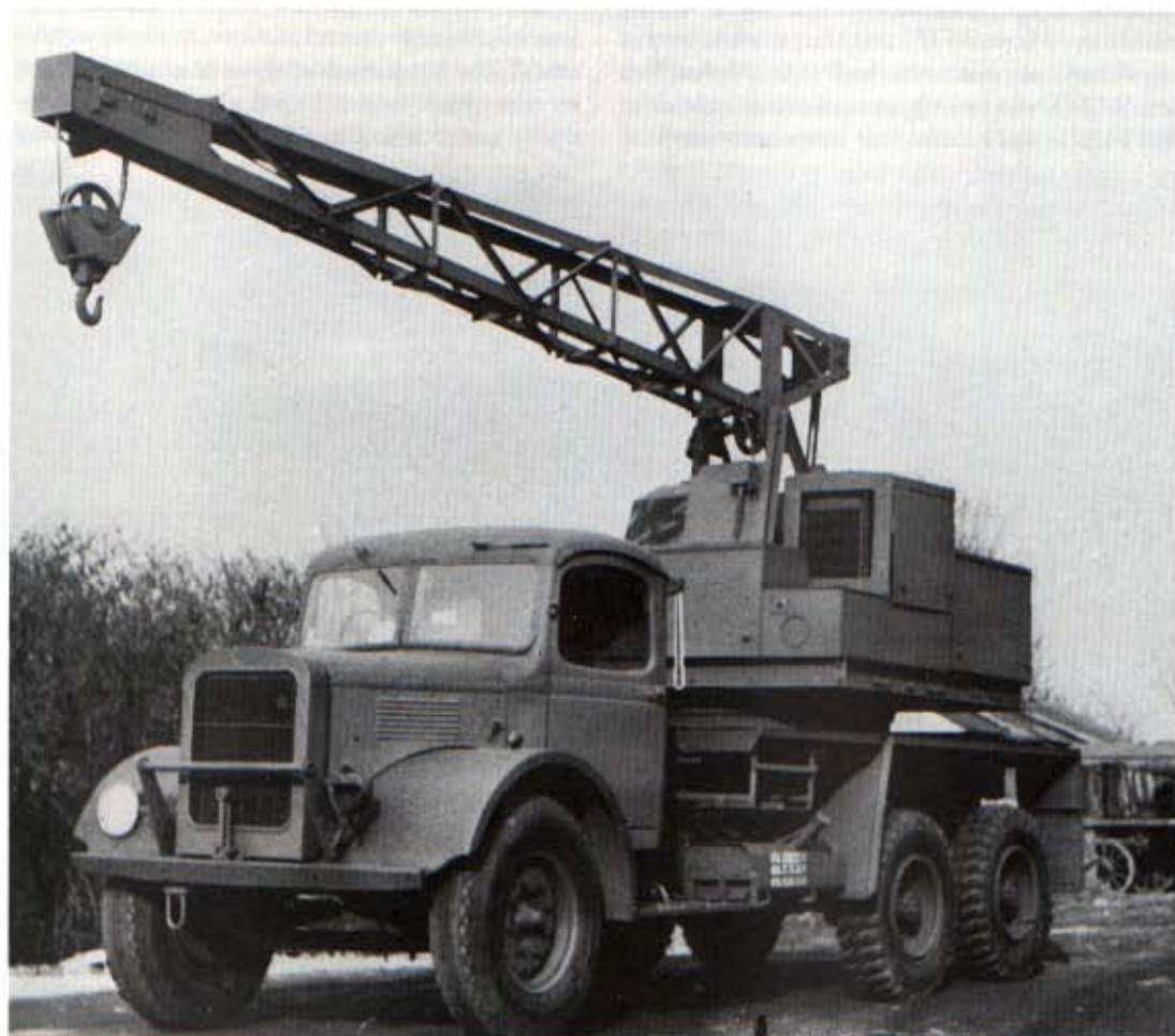
Above: Another popular chassis for crane carrying was the Thornycroft Amazon, which, like the AEC, used a Coles Mark VII. About 2000 were made during the war, of which the RAF took 1800. (NMM)
