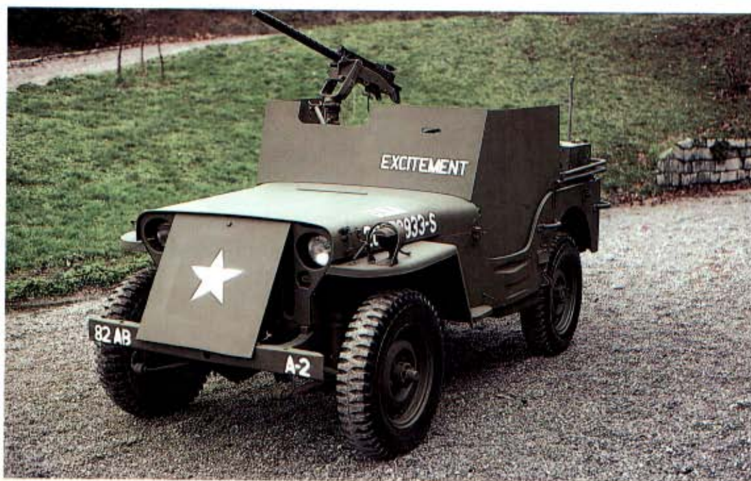
Left: The armour on this Jeep is a field modification. The lettering on the bumper indicates that it was used by the 82nd Airborne division, Company A, vehicle number 2. (Vehicle displayed at the Victory Memorial Museum)
