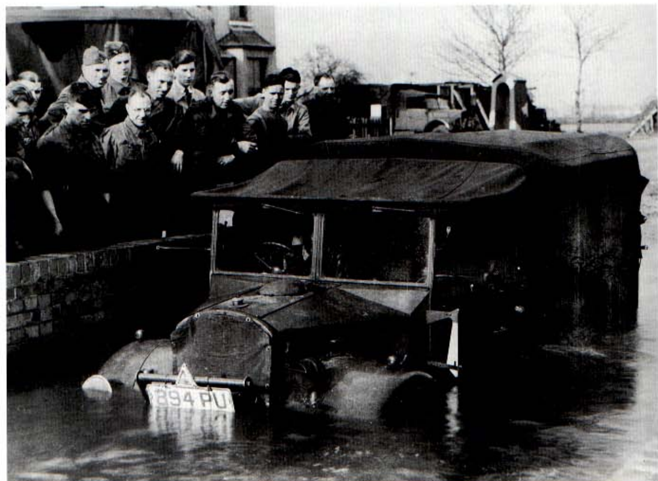
Above: Fordson WOT2E undergoing water-proofing tests under the watchful eyes of soldiers who might soon be depending on its water reliability. A total of 59,498 of the WOT series was made between December 1939 and December 1945.
