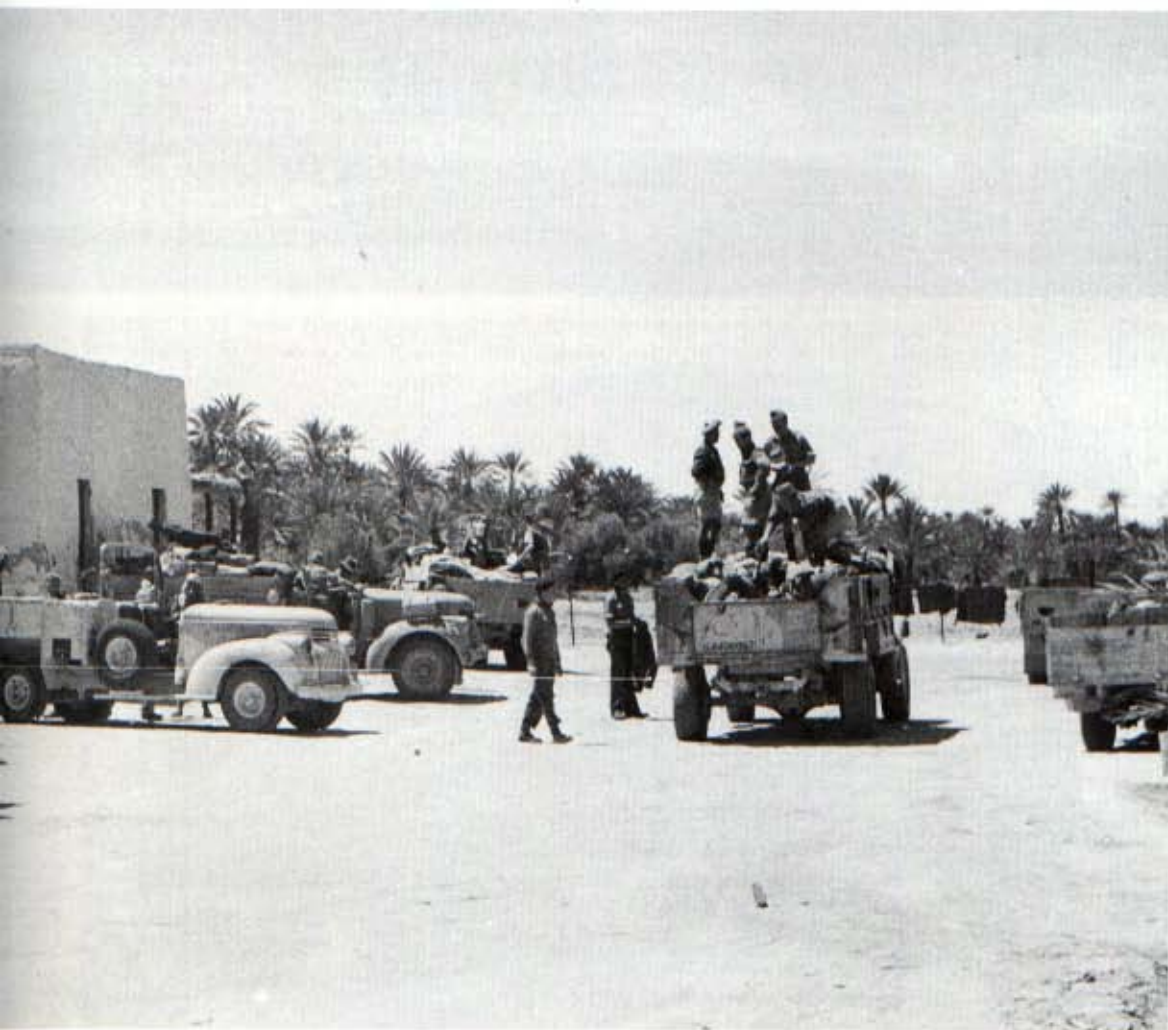
Left: Chevrolet 30 cwt trucks with Gotfredson ammunition-carrying welded bodies, used by the Long-Range Desert Group. This was a unit of the British Army formed in Egypt in 1940 to operate behind enemy lines. A patrol is about to leave the oasis which is the desert HQ of the LRDG. The nearest truck has had most of its grille removed for improved cooling. (JWM)
